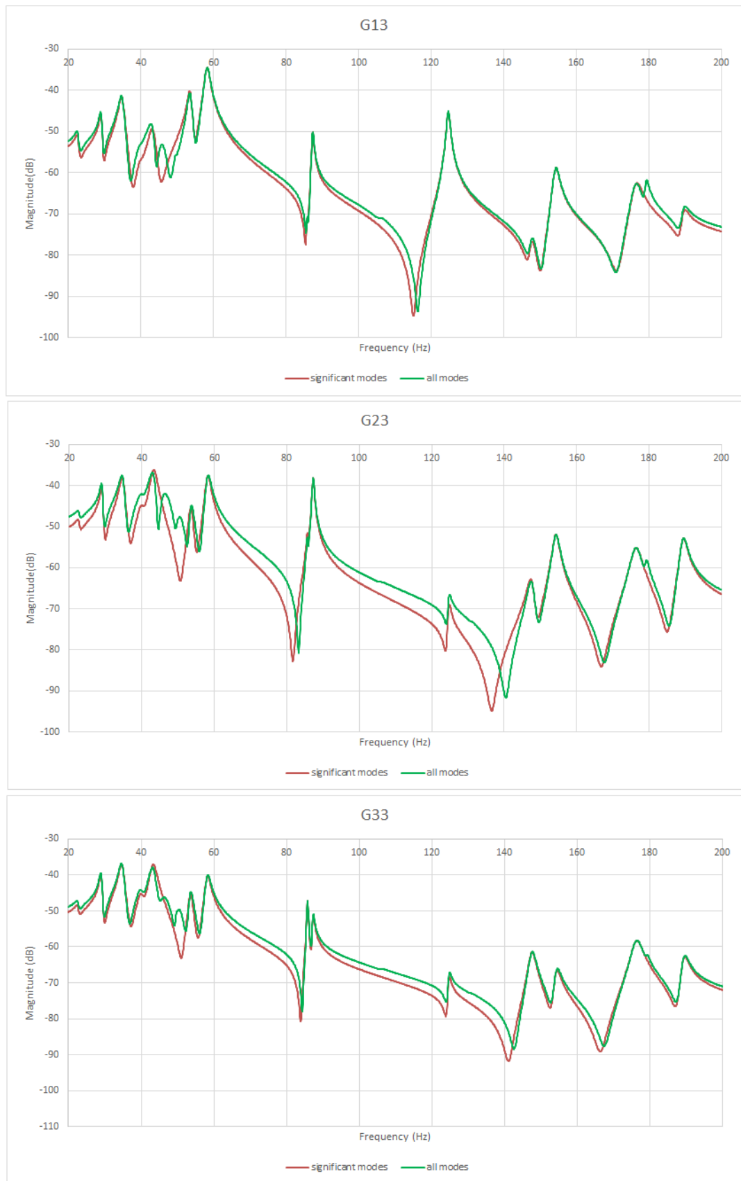
Figure 4.19 Comparison of FRF curves of all modes and significant modes-input from transducer 3
