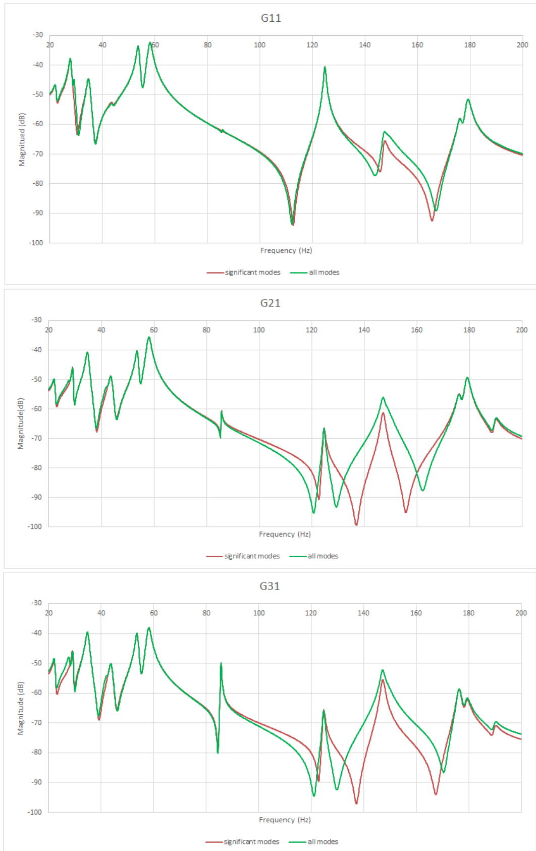
Figure 4.17 Comparison of FRF curves of all modes and significant modes-input from transducer 1
