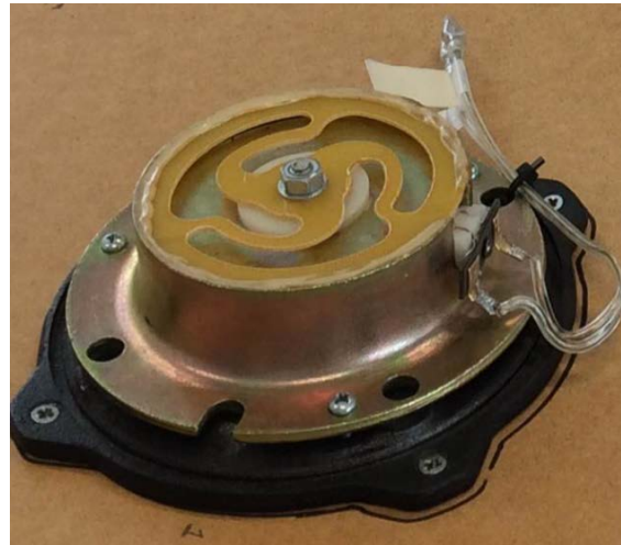
Figure 3.2 Electromagnetic transducer used as sensor and actuator
