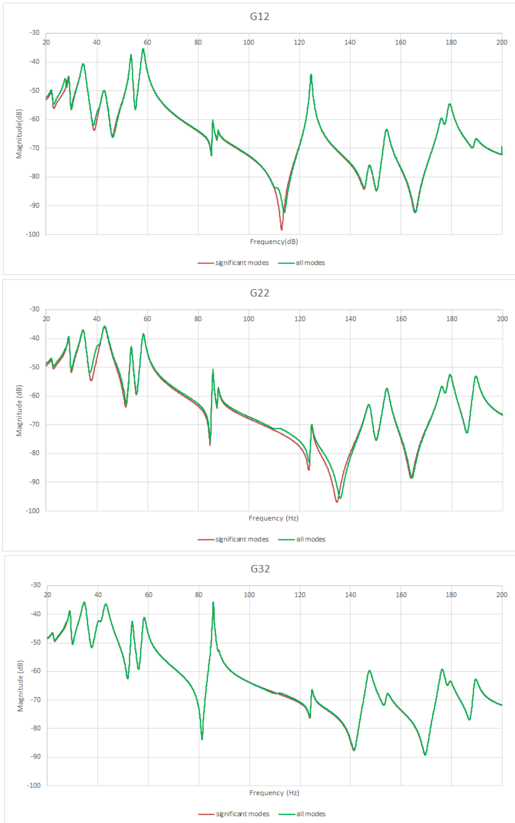
Figure 4.18 Comparison of FRF curves of all modes and significant modes-input from transducer 2
