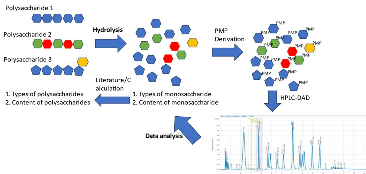
**Figure 2.5.1 Schematic diagram representing hydrolysis of polysaccharide and detection through HPLC analysis.**
