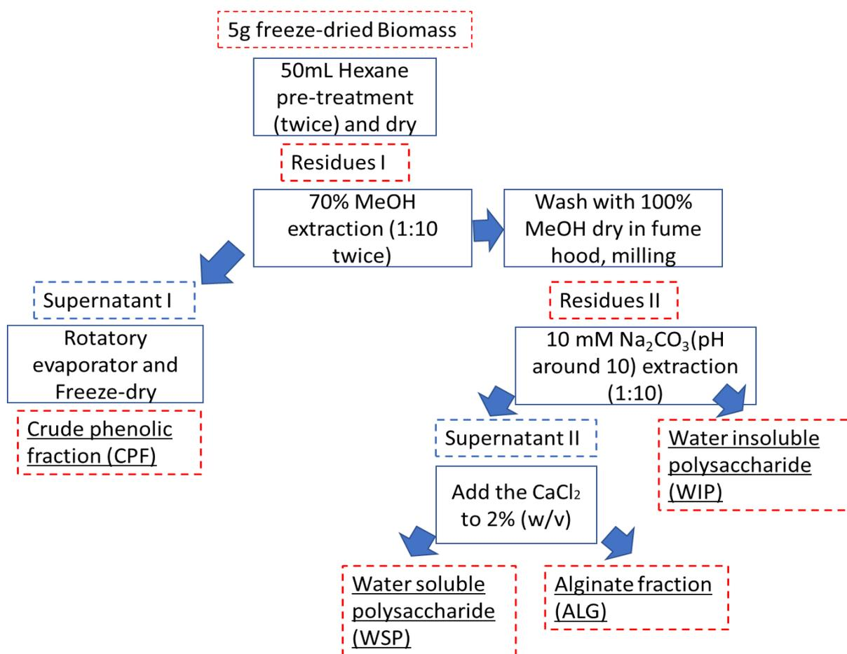
Figure 2.2 Layout of the process followed for extraction and purification of different fractions of leaf, stem, bladder and root.
