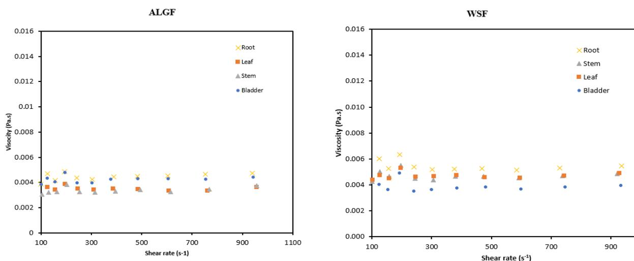
Figure 3.6 Flow curve of WSF and ALGF solution extracted from leaf, stem, bladder and root. The experiment was carried out using two technical replicates of each tissue used.
