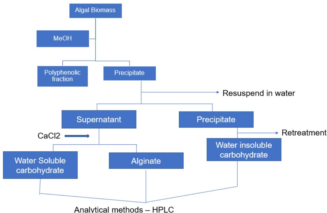
**Figure 1.3: Flow chart representing the general process of extraction and quantification of seaweeds bioactives**
