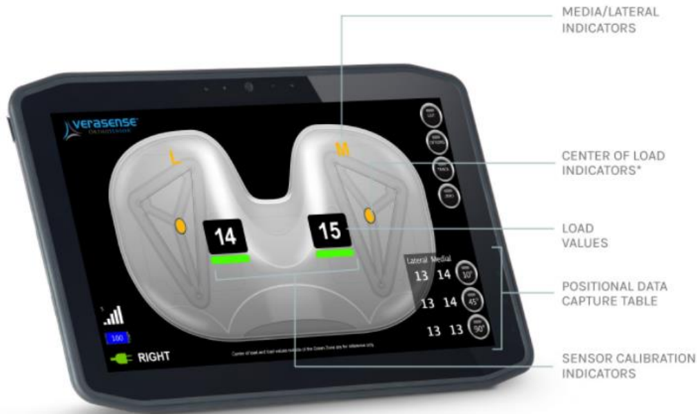
Figure 49: Live surgical display of tensions in the medial and lateral compartments of the knee. Reproduced with permission by Zimmer.
