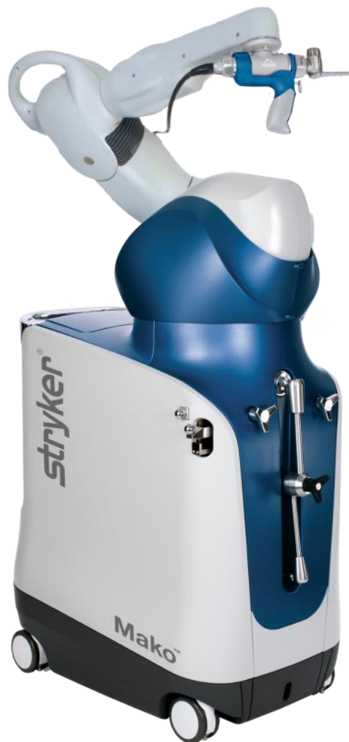
Figure 44 Example of surgical 'Robot' with its motorised arm for orientation of surgical tools in space. Reproduced with permission from Stryker 125
