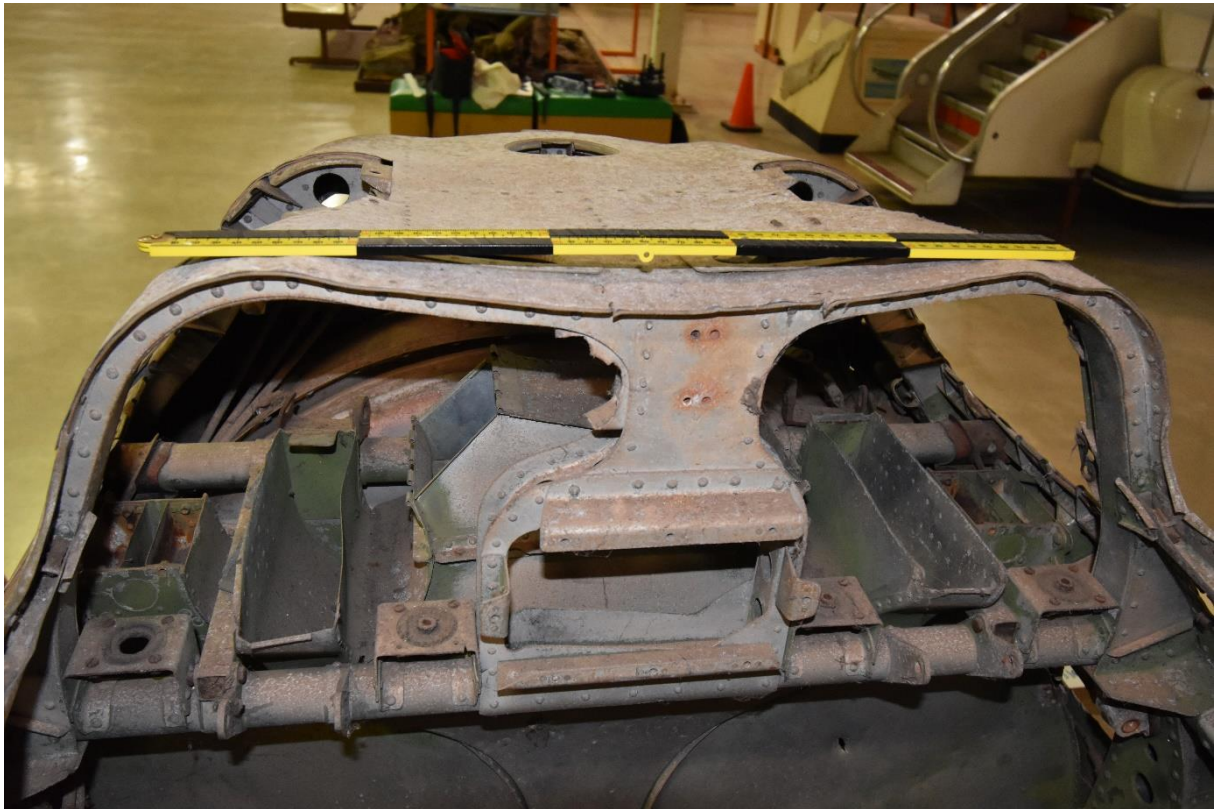
Figure 5.4. The top, front part of the cockpit, where a gunsight was mounted (Photograph: Author, 2 December 2021).
