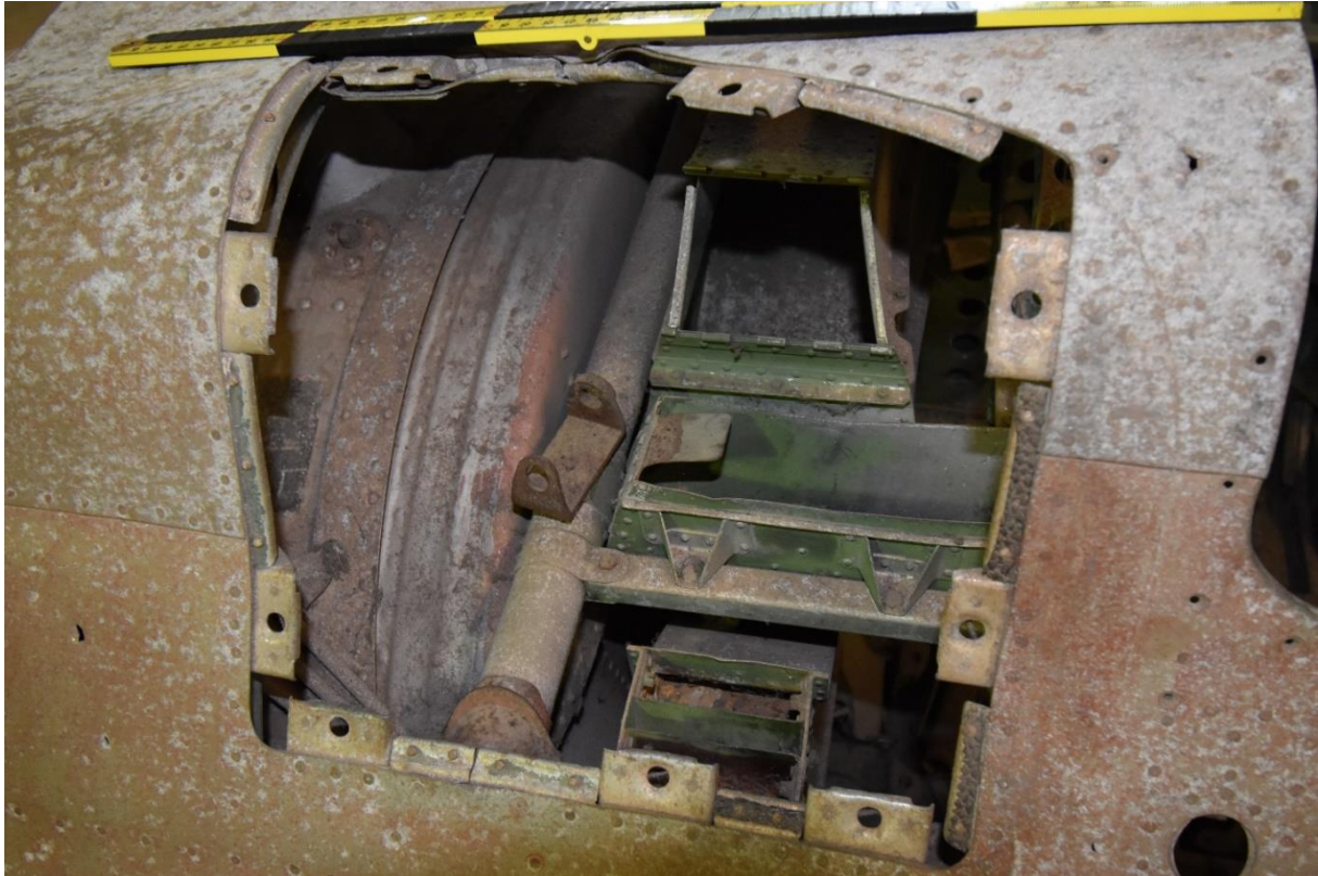
Figure 4.5. View of the main fuel tank (left), a front machine-gun mount (middle), cartridge ejecting tube (right) and machine-gun magazine (bottom) from the port side (Photograph: Author, 2 December 2021).
