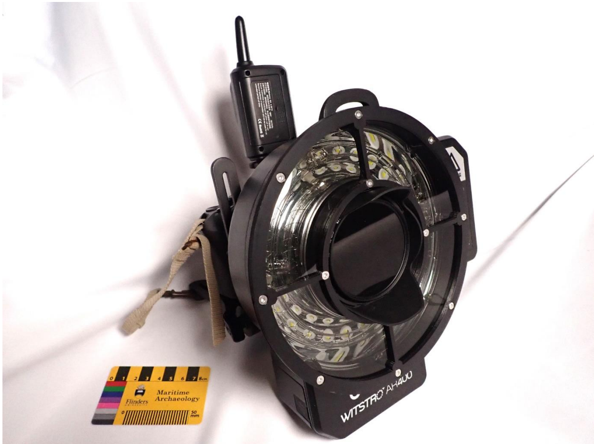
Figure 3.3. Camera configuration for the linear polarising filters method (Photograph: Author, 2022).
