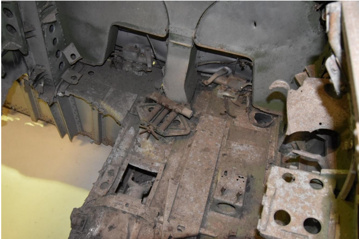
Figure 4.17. The inside cockpit view from the starboard side. The stem portion of the rudder bar adjustment mechanism is in the middle (Photograph: Author, 2 December 2021).
