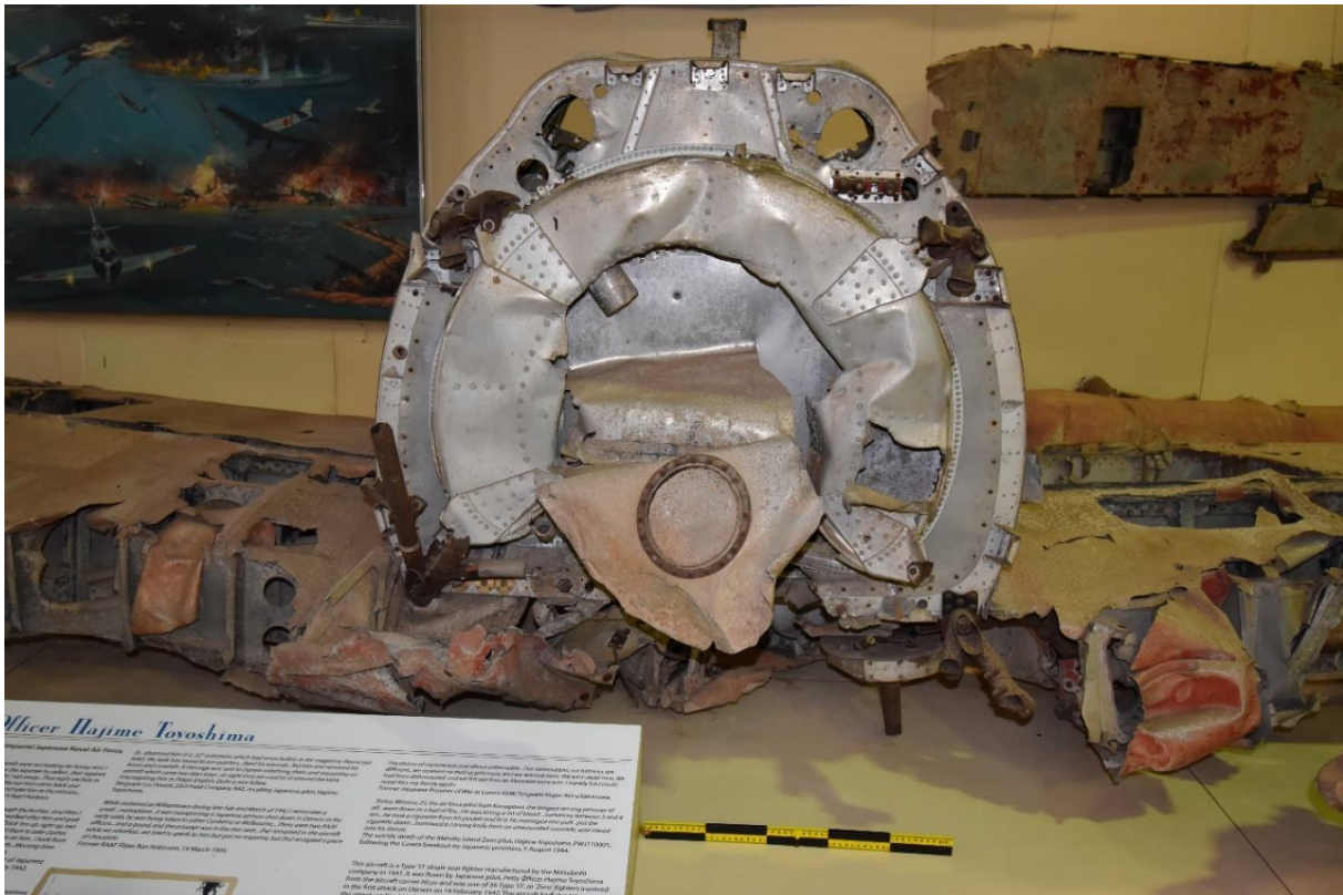
Figure 4.15. The view of the oil tank and remaining portions of the engine mount from the front (Photograph: Author, 2 December 2021).
