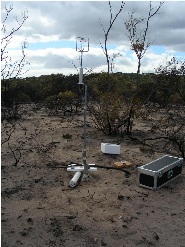
Ultrasonic anemometer in a recently burned site at Hincks Wilderness Protection Area, SA
