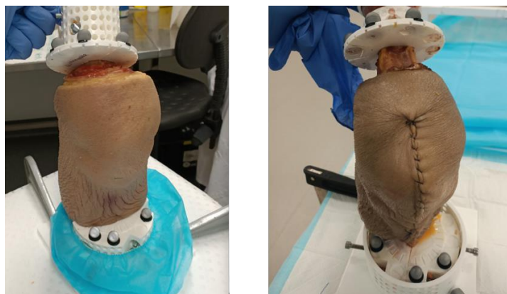
Figure B.1— Visual representation of a prepared intact and implanted knee specimen, featuring passive reflective markers for motion capture analysis, in accordance with the experimental setup and protocol outlined in Chapter 3 of the study.
