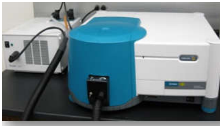
Figure 3.24: A photograph of photoluminescence spectroscopy model Varian Cary Eclipse with Peltier temperature controller and front surface accessory.
