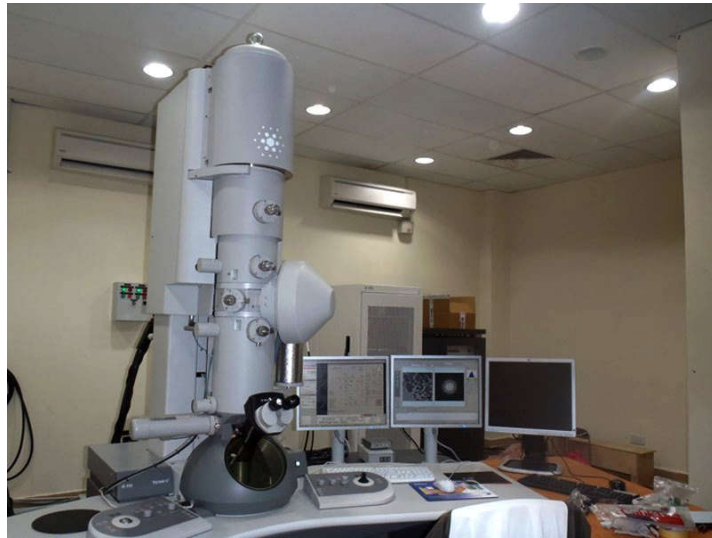
Figure 3.15: The HRTEM model Tecnai G2 20 S-Twin, FEI
