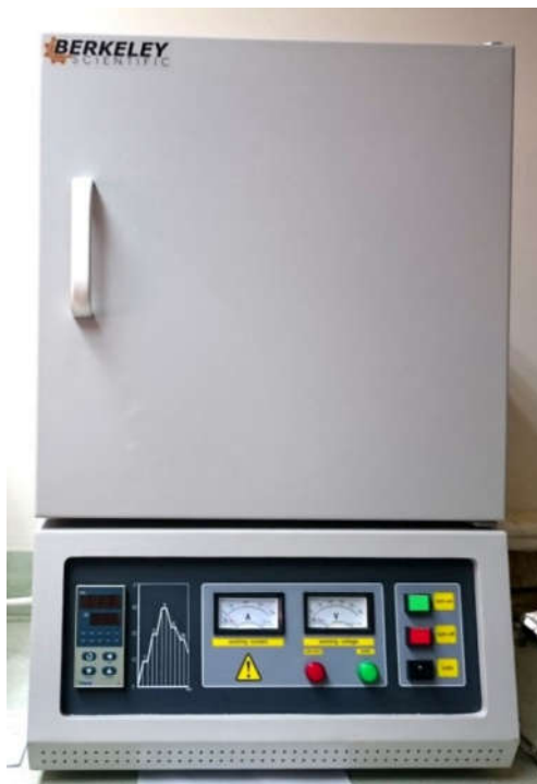
Figure 3.3: Electrical furnace model Berkeley-Scientific 1700 °C for melting process
