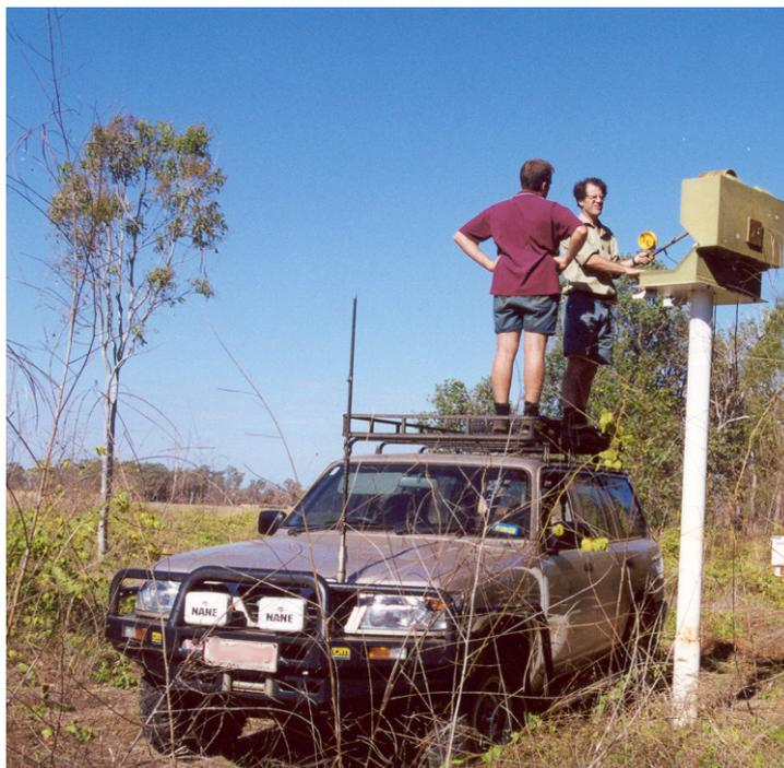
Figure 4.1: Wells with very tall standpipes are often constructed to avoid inundation by floodwaters. This example is from the Daly River, Australia (courtesy of Steven Tickell).
