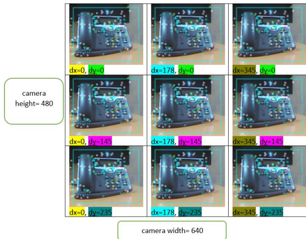
Figure 9 dx= h31 and dy= h32 values regarding to the object position in camera frame
