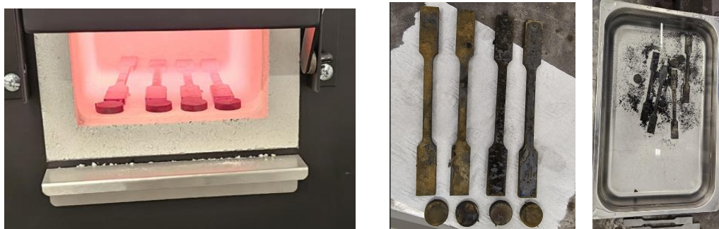
Figure 11: Quenching in water treatment process in furnace, and final results of the samples.
