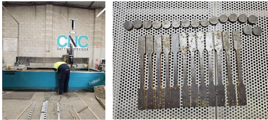
Figure 1 Water Jet Cutting machine and prepared sample by CNC Cutting services.
