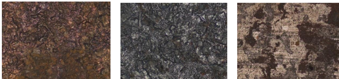
Figure 18: Quenching in water sample, sandblasting sample, Untreated sample
