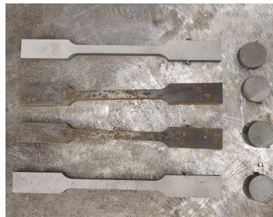
Figure 12: Untreated and sand blasted samples of tensile and hardness testing.
