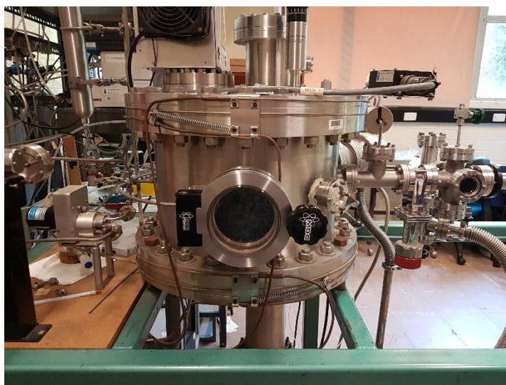
Figure 2-1: Plasma chamber used in this work.
