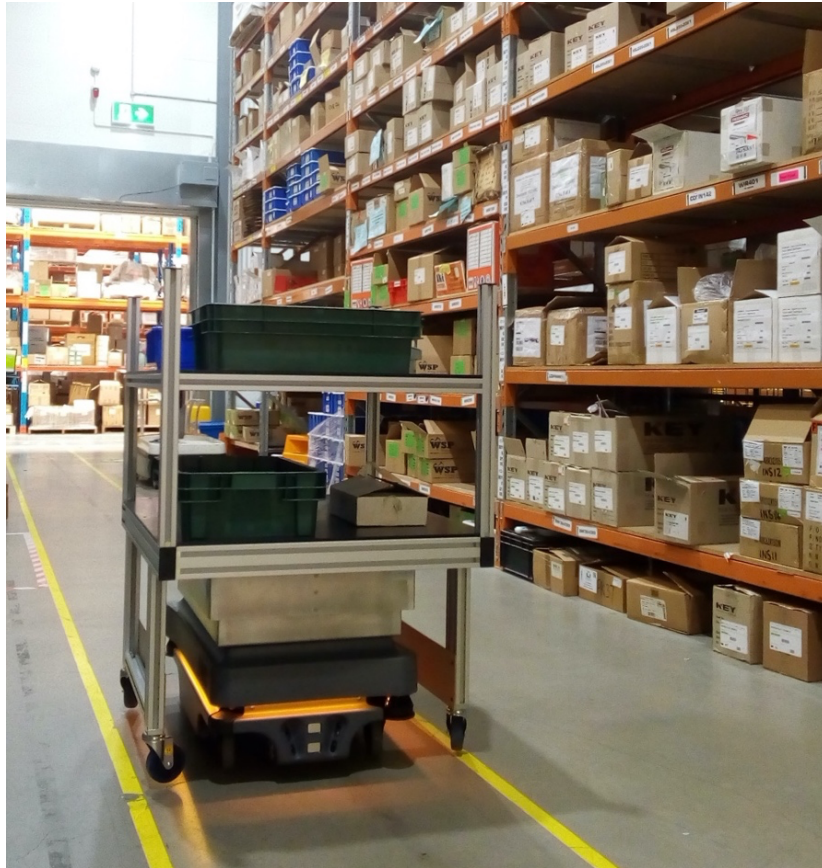
Figure 13: Mobile Robot and Trolley at REDARC
