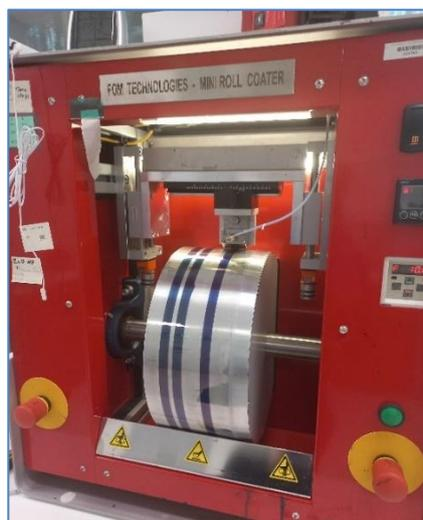
**Figure 3.9:** Image of the MRC used throughout the thesis. Included in the image of active materials being deposited from the slot-die coating head.
