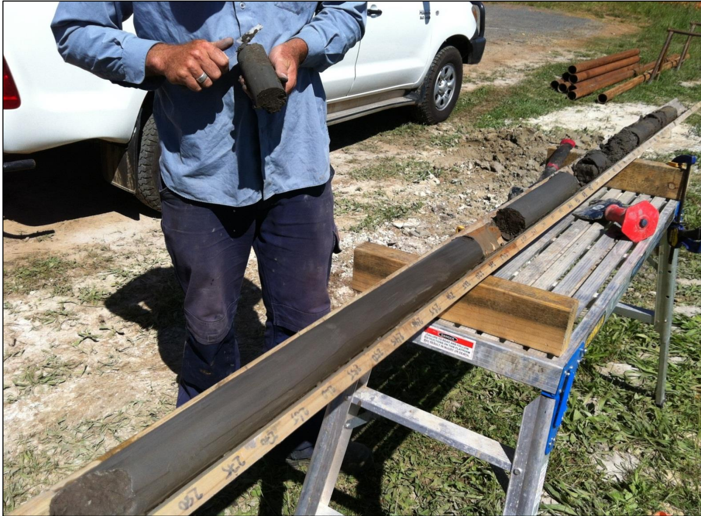
Photo 6: Core at Site 1. Core was placed in the jig by the drillers, we recorded the measurements, lithology and collected cores for scraping (shown), and sealing by vacuum sealing or for noble gas analysis.
