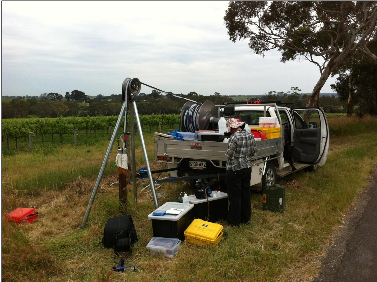
Photo 4: Groundwater sampling near the vineyards, this pump and winch was constructed to reach a depth of 200m.
