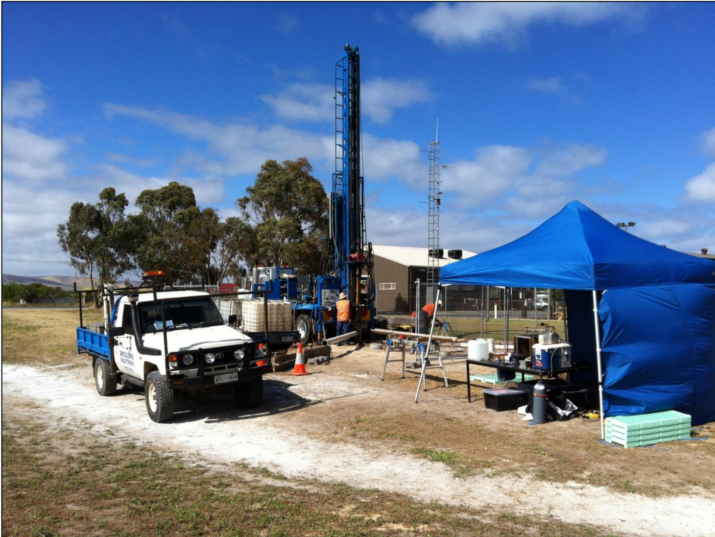
Photo 5: Aquitard coring and sampling at Site 1 (Aldinga) on a 40°C day.
