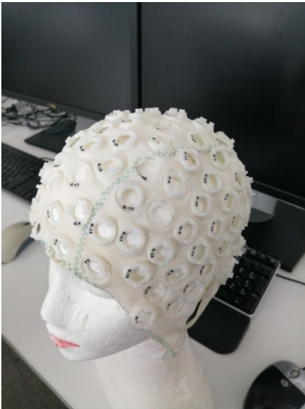
Figure 32. Size 58 EasyCap used for Experiment 3 on a dummy head model.
