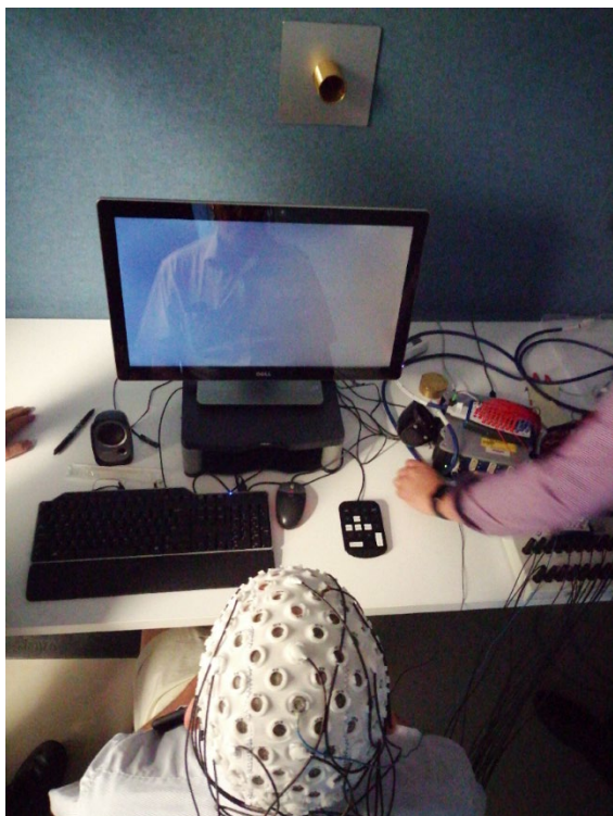
Figure 24. Participant being prepared for experiment start. Devices being powered up for the start of the experiment. Pad on right side of keyboard for stimuli response.
