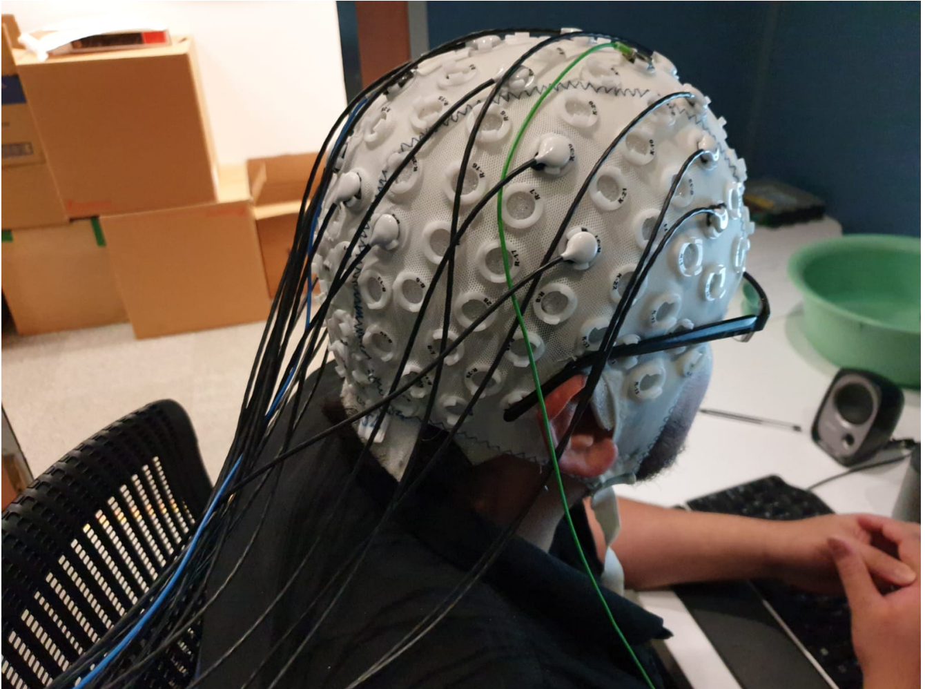
Figure 30. Subject with thick hair with the foam cap under the tCRE cap. The electrode holders under the tCRE electrodes have foam fillings (black bits sticking out) filled with saline.
