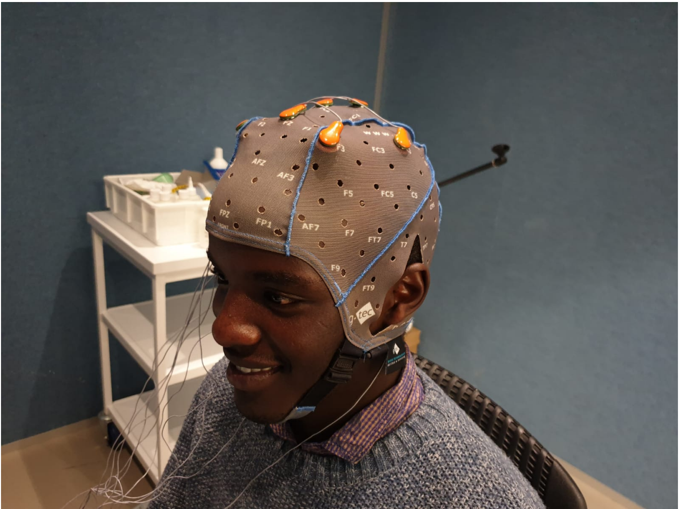
Figure 37. Subject with short, stiff, curly hair with the SAHARA electrode gtec cap fit on
