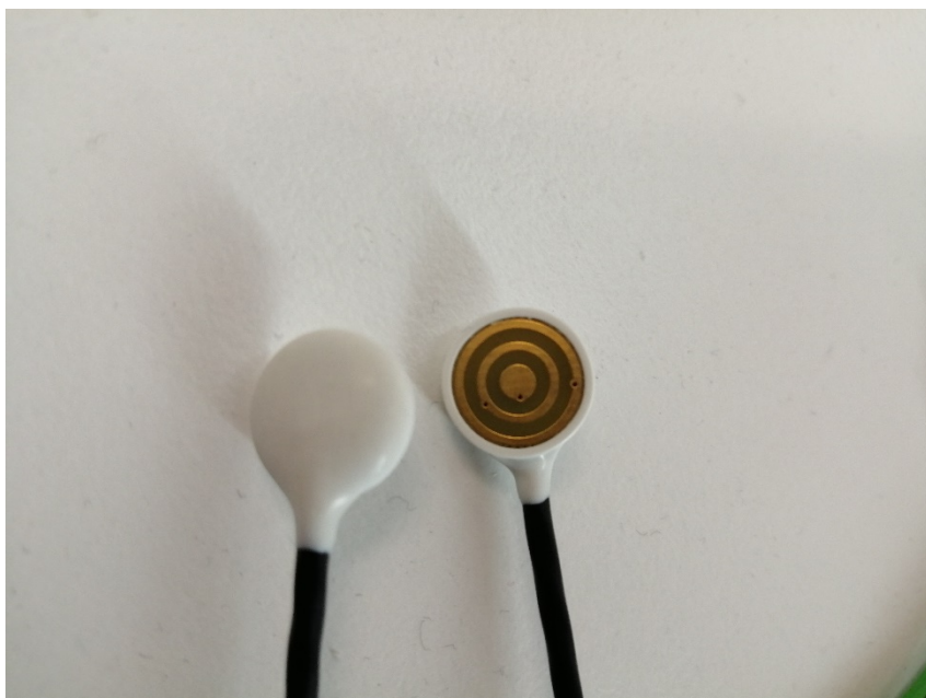
Figure 10. tCRE electrodes used for experiments. 2 rings (gold) visible in image concentric around central disc
