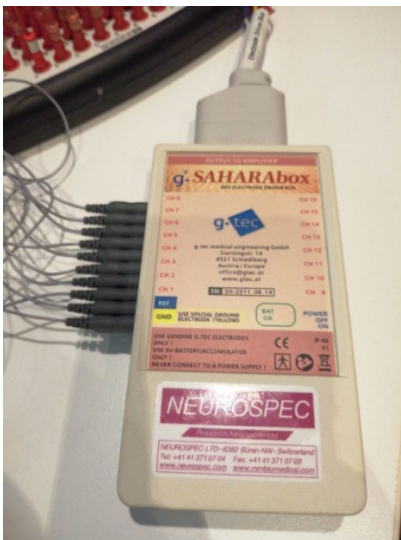
Figure 35. 16 channel SAHARA electrode headbox, with incoming electrode connectors (black) and outgoing channel to the Hlamp (white)
