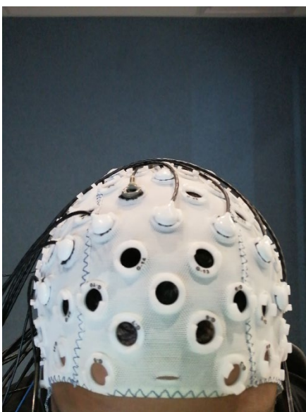
Figure 29. Test 2 run with author as participant to verify effect of hair volume on interface connection quality
