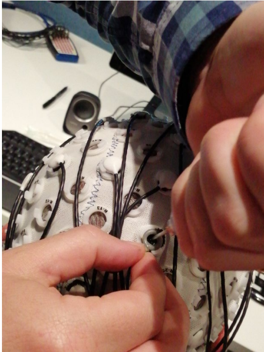
Figure 28. Application of saline to the foam placed in the space in a ring electrode, used as reference/ground in experiment 4
