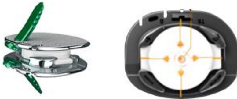
Figure 43: An assembled MobiDisc-L TDR (left) and the mobile core of the MobiDisc-L that allows semi constrained translation in the transverse plane and axial rotation(right) (Zimmer Biomet 2016).
