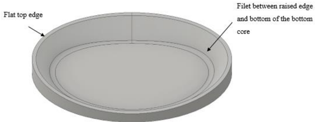
Figure 77: First design iteration with flat top edge and fillet between raised edges and bottom of the bottom core.
