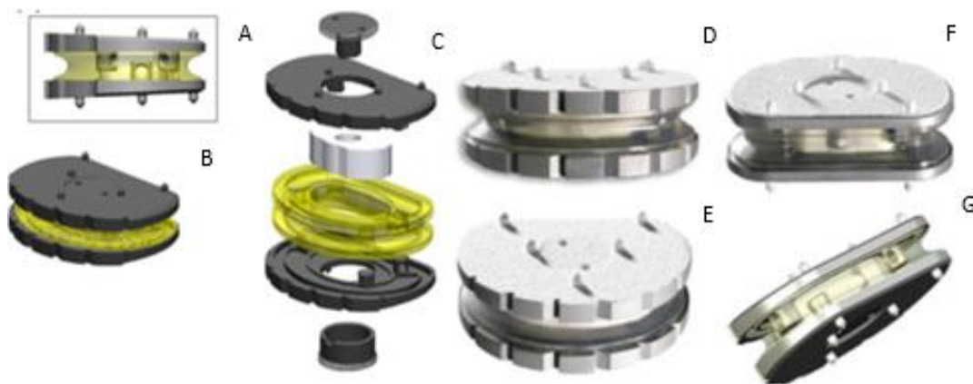
Figure 48: CAD exploded view showing the LP-ESP inner silicone gel core and polycarbonate urethane ring (A-C). The actual LP-ESP TDR with titanium endplates and five spikes for fixation (D-G)(Lazennec et al. 2012).
