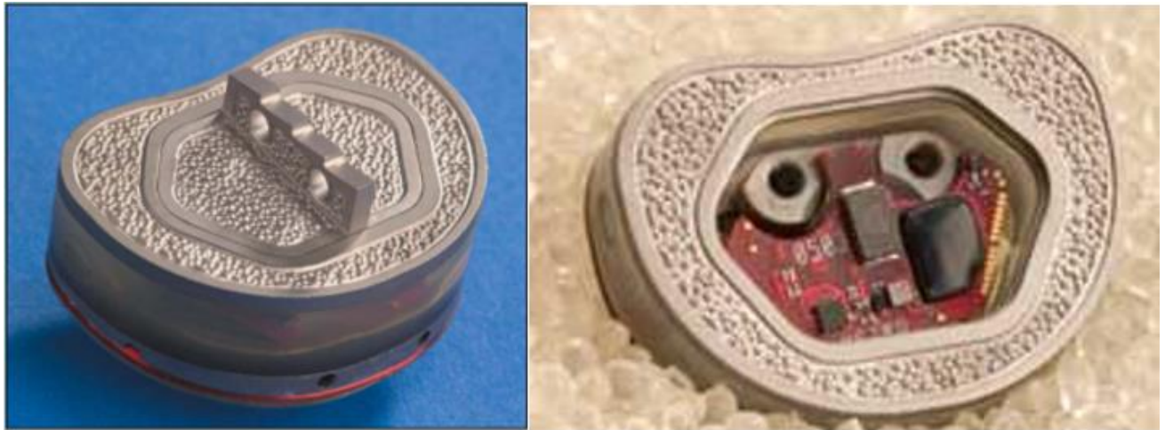
Figure 32: Assembled eDisc TDR (left) and eDisc with exposed electronics (right)(Hunt et al. 2007)(McMillin 2006).
