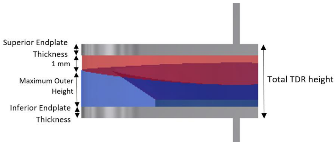
Figure 88: The maximum outer height of the bottom core = Total TDR height - 1 mm - Superior Endplate Thickness - Inferior Endplate Thickness.
