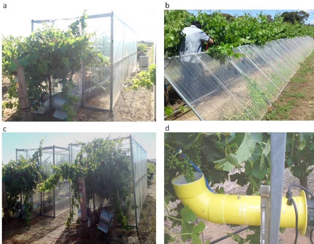
Figure A.1.4. Equipment used for heat treatment of vines in the field. Single, closed chambers (a) were used for 3 days at a time, open-top chambers (b) were assembled for 3 weeks at a time, while “control” and “heated” closed chambers (c), each containing “control” and “heated” bunch blowers (d) were assembled for 10 days at a time.
