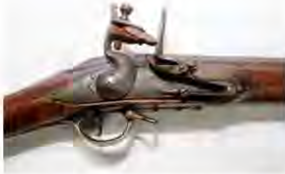
Figure 4 India Pattern 'Brown Bess' musket. Shown is the flint striking the frizzen above the pan to cause a spark igniting the powder in the pan and chamber to discharge the shot. The unreliable action coined the phrase 'a flash in the pan' (image courtesy < https://goo.gl/images/BQxMP2 >).
