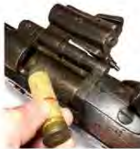
Figure 41 Loading a Boxer cartridge of rolled sheet brass construction into the Jacob Snider Jnr designed hinge-block breech loading action of a Snider-Enfield rifle, the precursor to modern-day breech loading and centre-fire cartridge ammunition weapons (image by Tony Pagels).
