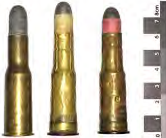
Figure 67 Left to Right. (Left) Boxer-Henry brass drawn rifle cartridge, in use from 1885; (Centre) Boxer -Henry rolled brass rifle Eley 'Contract E', in use from 1888 with white paper patch and 85/480 grain charge and bullet, without inspection hole; (Right) Boxer-Henry rolled brass carbine cartridge Mk III and in use from 1879 with red paper patch and 70/410 grain charge and bullet, with inspection hole. The brass drawn carbine cartridge (not pictured) was introduced in 1887 (Temple 1977:88, 93-96) (image by Tony Pagels).
