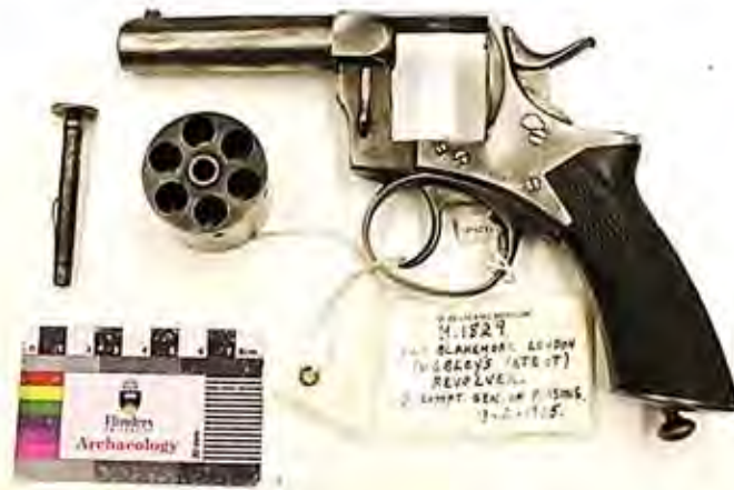
Figure 54 Webley R.I.C. No.3 first pattern serial number: 6787. Removing the arbor (pin holding the cylinder to the frame) releases the cylinder for loading and unloading, and the handle is made of a single piece of chequered walnut without the horn projection. This revolver is held at the Queensland Museum collection no. H1829 refers (image by Tony Pagels).
