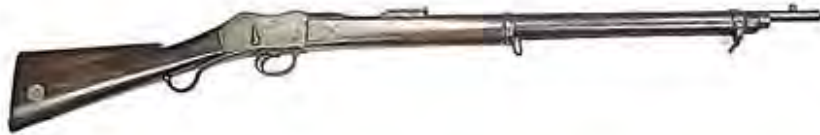
Figure 62 Martini-Henry rifle Mk I converted to Mk II Pattern and marked on the right-side receiver with the Royal cypher over Enfield 1874 II along with Q†G 7749. The right side of the butt is stamped Q†G 7749, the makers mark and 1901. This arm is held in the Queensland Police Museum collection (image by Tony Pagels).
