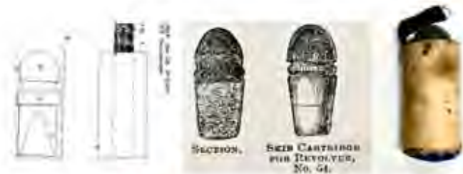
Figure 32 (Left) Detail of bullet and paper cartridge design from the patent drawings for William Eley's paper revolver cartridge Patent 2487 dated 24 November 1854. (Centre) Tranter revolver .442 calibre (54 bore) skin cartridges as advertised on an Eley Bros flysheet circa 1859/1860. (Right) Tranter cartridge with blue base marked Eley London (images courtesy of [left] English patents of inventions, specification: 1854, 2471 –2520 [centre] Harding 2006:124, [right] Tony Pagels).
