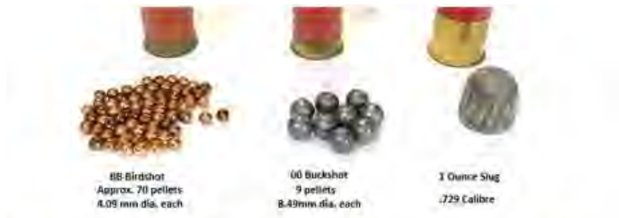
Figure 38 A visual comparison of various sized projectiles for a 12-gauge shotgun cartridge (image by Tony Pagels).
