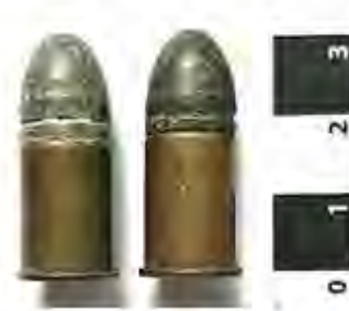
Figure 49 Examples of .442-inch cartridges produced by Eley Brothers (left) post 1874 and (right) pre 1874 after the formation of Eley Brothers Ltd. Note the slight variations in the case crimping, cannelure and bullet definitions (image by Tony Pagels).
