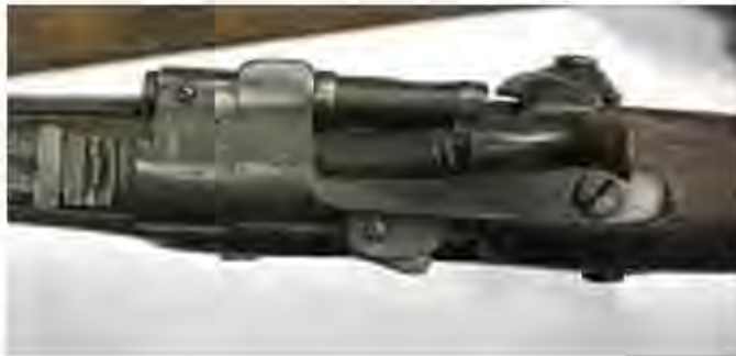
Figure 42 Snider artillery carbine MkIII depicting the closed hinged block breech. The MkIII is fitted with the spring-loaded locking latch, on the left side of the block. This Snider artillery carbine is held in the Queensland Police Museum collection (image by Tony Pagels).
