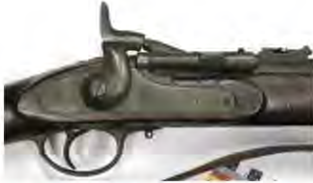
Figure 58 Snider artillery carbine MkIII without sword bar and full steel furniture. Detail of the lockplate marked P. WEBLEY & SON over LONDON & BIRMM over 1874 below the breech and stamped † over QP on the lockplate behind the hammer. This weapon is also stamped † over QP in the timber on the right of the butt. This Snider is held in the Queensland Police Museum collection and a second example of a Snider artillery carbine stamped in this manner is held in the Queensland Museum collection no. H1351 refers (image by Tony Pagels).
