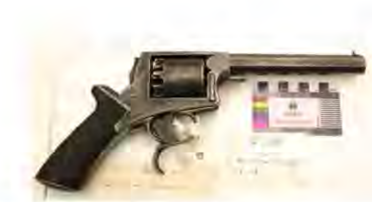
Figure 30 An example of a Tranter double trigger, 54 bore percussion revolver. Immediately obvious are the two triggers along with the absence of a spur on the hammer. This revolver is held in the Qld Museum collection H2227 (image by Tony Pagels).
