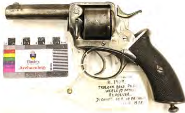
Figure 51 Webley R.I.C. No.3 Second Pattern six-shot revolver. This revolver is from Trulock Bros. and not numbered. The 'No.3' features include the removable arbor and the arbor release mechanism. The 'second Pattern' features included the projection or horn and the butt, which is made of two pieces of chequered walnut and the raised cylinder bolt projections at the rear of the cylinder. The frame is marked "C.I.B. 1005", and ↑ over Q.G. This revolver is held at the Queensland Museum collection no. H1909 refers (image by Tony Pagels).
