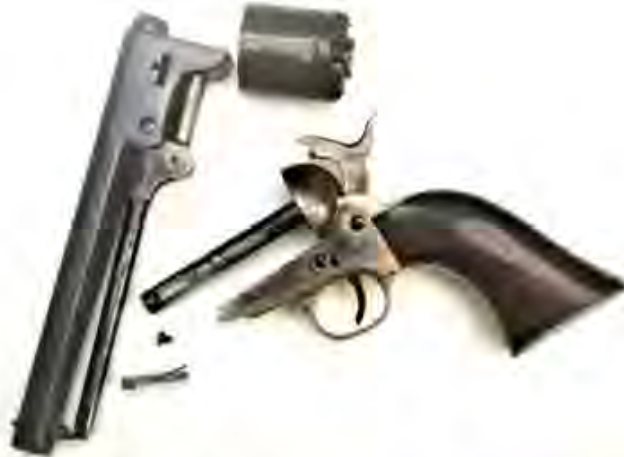
Figure 18 A dismantled Colt Navy, demonstrating the simple construction, with parts easily interchanged (image courtesy of Prescott (2013:27).
