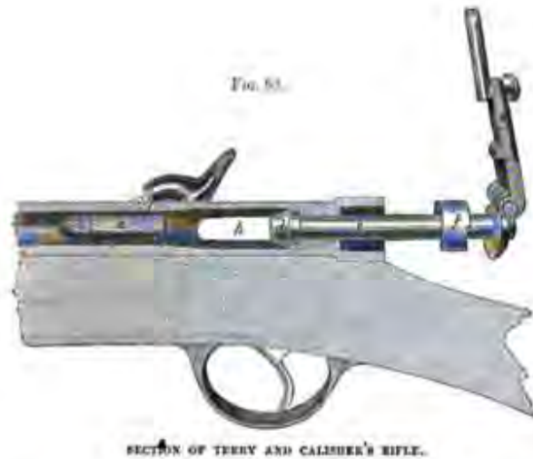
Figure 12 Section diagram of the Calisher & Terry capping breech-loader with the bolt withdrawn to show the cartridge in the chamber. The paper cartridge is loaded from the right side through the opening marked 'h' and the gas-tight seal is achieved when the stopper, 'd', is locked in place (Walsh 1859:333).
