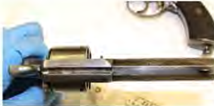
Figure 55 Webley R.I.C. No.3 first pattern six-shot revolver serial number: 6787. This image depicts the top strap marked with the name "V&R BLAKEMORE LONDON". The cylinder is smooth, apart from the bolt slots can be seen at the front of the cylinder. Visible on the right side behind the cylinder is the protruding latch to load the cylinder via a swinging gate, an adaption from the No.1 First Pattern. This revolver is held at the Queensland Museum collection no. H1829 refers (image by Tony Pagels).
