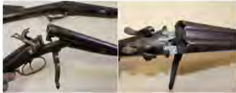
Figure 35 Westley Richards & Co. breech loading double barrel carbine, 20g with Lefauchaux-action. The action is open to illustrate the design of the drop breech and slot in the top of the barrel to accommodate the pin of the cartridge. With the breech closed the pin protrudes into the slot and on being struck by the falling hammer is pushed inward igniting the percussion cap and power to discharge the bullet (images by Tony Pagels)
