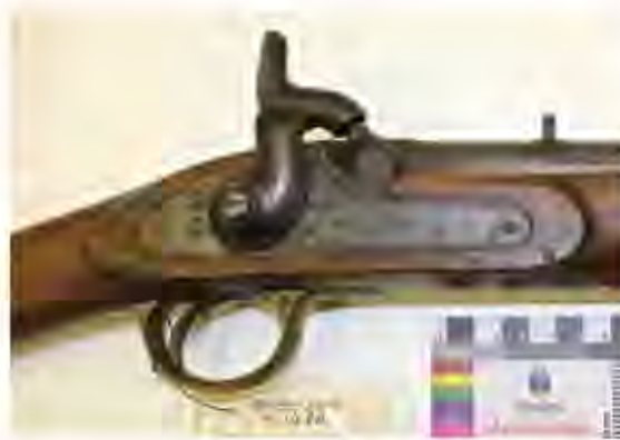
Figure 5 Potts & Hunt single barrel percussion carbine. A percussion cap is placed over the nipple and struck by the hammer causing a spark to ignite the powder in the breech. The carbine is from the Queensland Museum collection catalogue number: H1480 (image by Tony Pagels).
