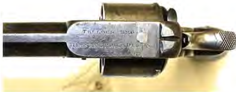
Figure 52 Depicts the top strap of the Webley R.I.C. No.3 Second Pattern six-shot revolver in Figure 51 marked with the name 'TRULOCK BROS. 11 ESSEX BRIDGE DUBLIN'. The cylinder is smooth and visible on the right side behind the cylinder is a protruding latch to load the cylinder via a swinging gate. The raised cylinder bolt projections can be seen at the rear of the cylinder. The top of the loading gate is on the right behind the cylinder. This revolver is held at the Queensland Museum collection no. H1909 refers (image by Tony Pagels).
