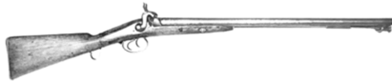
Figure 6 Double barrel 20-gauge cavalry carbine also known as the 'Cape' pattern carbine with the trumpet bracket for the ramrod and the scrolled trigger guard extension (Robinson 1997:17) (image courtesy of Skennerton 1975:76).
