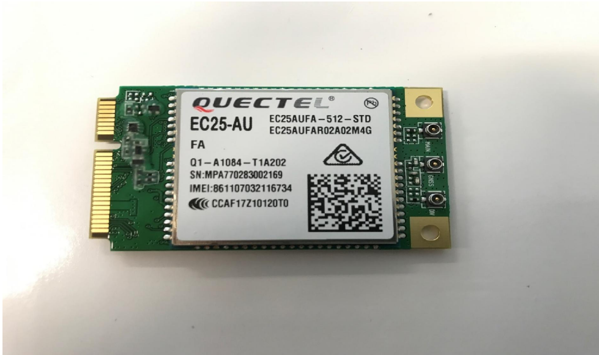
Figure 43: The EC25AUFA-512-STD (4G LTE) module by Quectel
