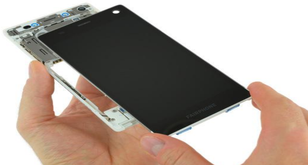
Figure 15: Sliding mechanism for separation of display from mainframe (ifixit, 2015).
