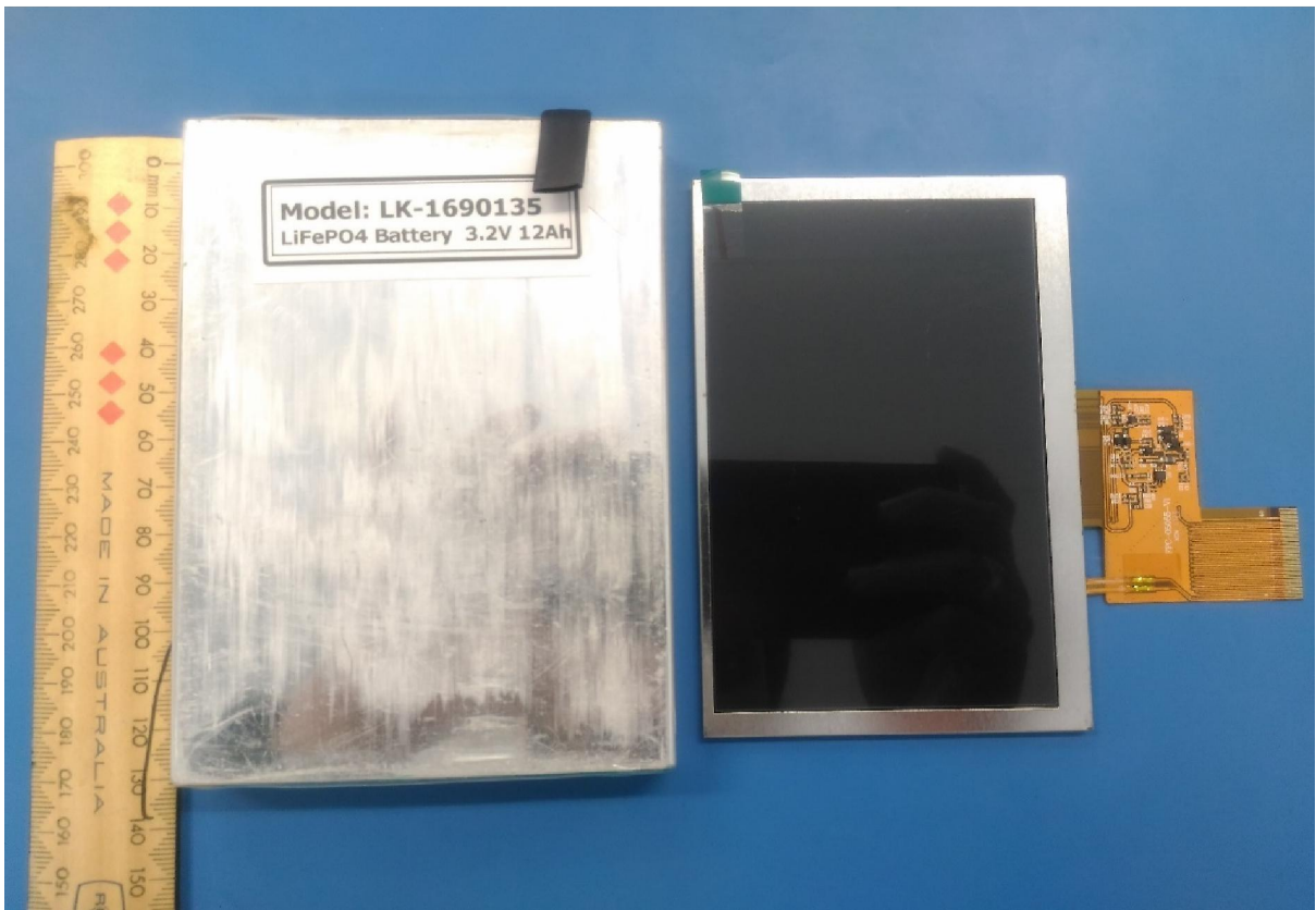
Figure 45: Comparing the dimension of LCD panel with LiFePO4 battery
