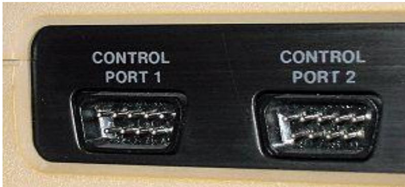
Figure 54: Control port (9-pin) for joystick connection (C64 Wiki, 2016).
