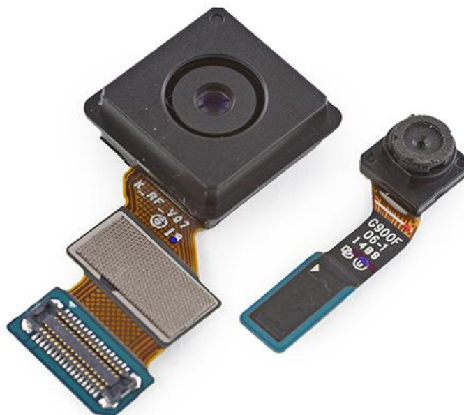
Figure 5: Samsung Galaxy S5 camera module with f/2.2 lens and Samsung S5K2P2XX1/2.6" sensor (Schiesser, 2014).
