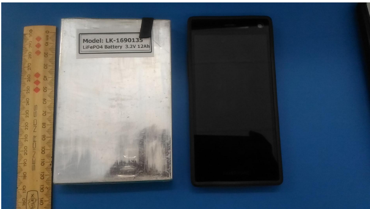
Figure 49: Comparing battery dimension with smartphone (Fairphone 2) as reference
