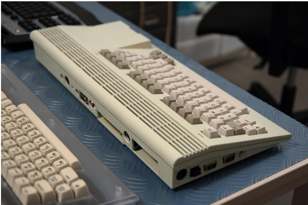
Figure 4: Side and Rear view of Commodore 65 with various peripherals connection slot (Detlef Hastik et al., n.d.).
