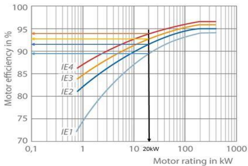
Fig 4 Efficiency standard for 4-pole, 50Hz low voltage electric motor [7].
