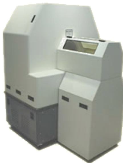
Figure 4.1: Siemens MicroCAT-II micro-Computed Tomography scanner.
