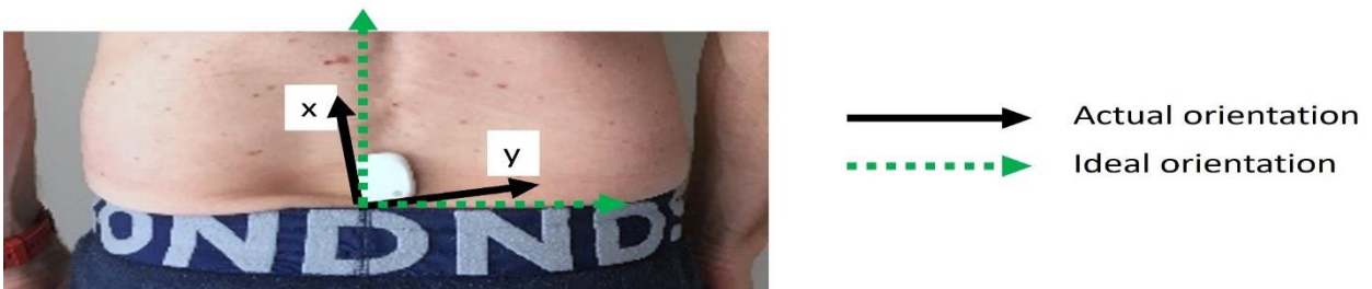
Figure 16: The positioning of the accelerometer on the lower back. The sensor's actual LCS is highlighted in black, while the target LCS is represented with dashed green lines.
