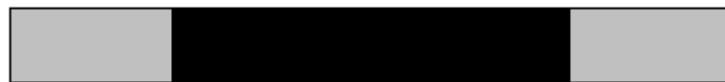
Fig 1.29: Depiction of a nanorod with discrete surface regions that are each compatible with different microphases of a block copolymer.
