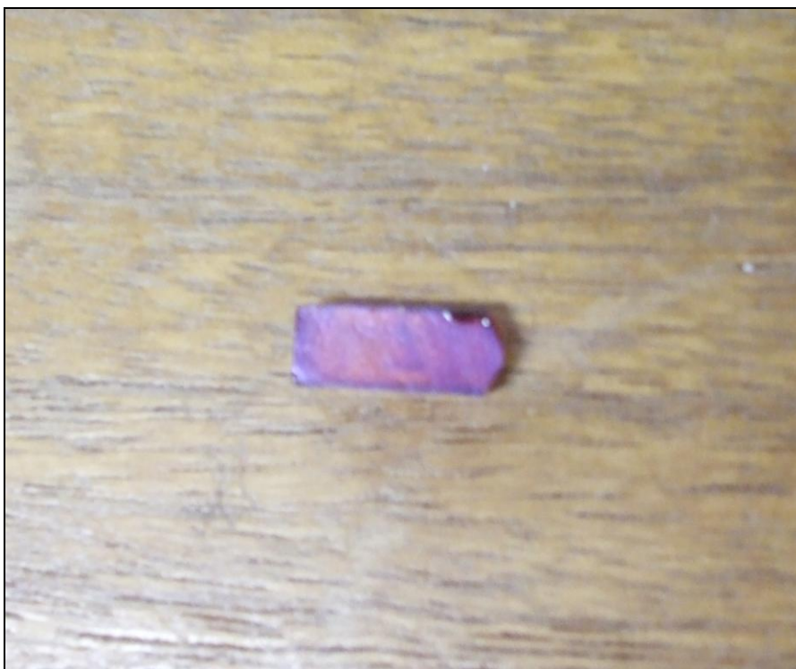
Fig 2.11: Image of an iodine stained, microphase separated PS-b-P2VP film (lamellar morphology) on an epoxy substrate.
