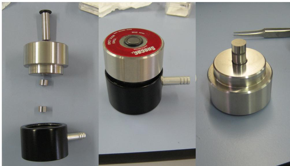
**Figure 34 – Left Panel: The die cast and its components. From top to bottom: Plunger, chamber, upper end cap, lower end cap and the base. Centre Panel: The assembled die cast. Right Panel: The base is removed and the cast inverted to push the pellet out of the chamber.**
