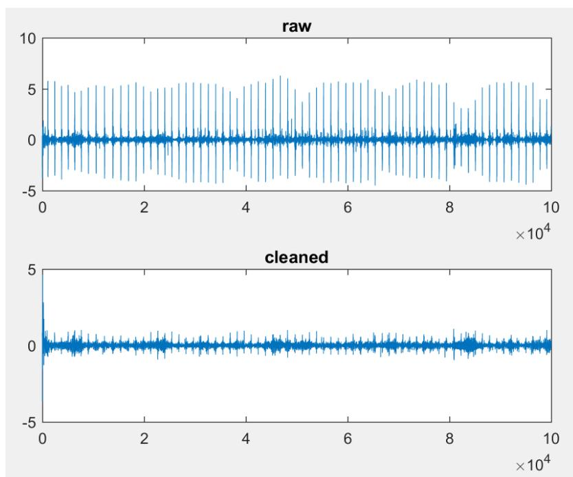
Figure 30 Channel 1 using ICA-Wavelet filter
