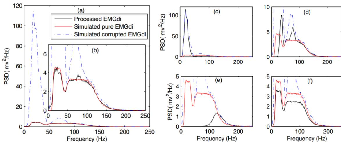
Figure 18 Signals comparison of PSD: (a) Wavelet-based adaptive filter result (b) expanded scale (c) Hard threshold result (d) 'inverse' hard threshold result (e) High pass filter result (f) gating technique result
