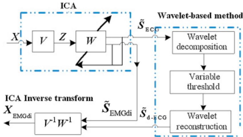
Figure 22 The block chart of ICA-Wavelet algorithm (Wu, Tong & Yang 2016)
