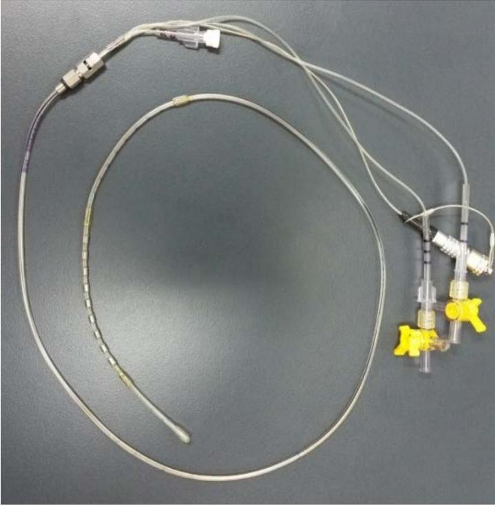
Figure 7 Esophageal catheter used in the Lab
