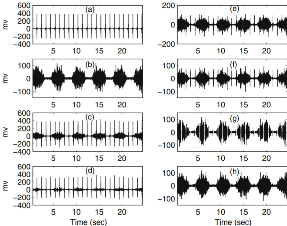
Figure 16 Signals comparison: (a) The ECG artifact signal (b) The pure EMGdi signal (c) The corrupted EMGdi signal (d) Hard thresholding result of EMGdi (e) 'Inverse' hard thresholding result of EMGdi (f) High pass filter result of EMGdi (g) Gating technique result of EMGdi (h) wavelet-based adaptive filter result of EMGdi (Zhan, Yeung & Yang 2010)
