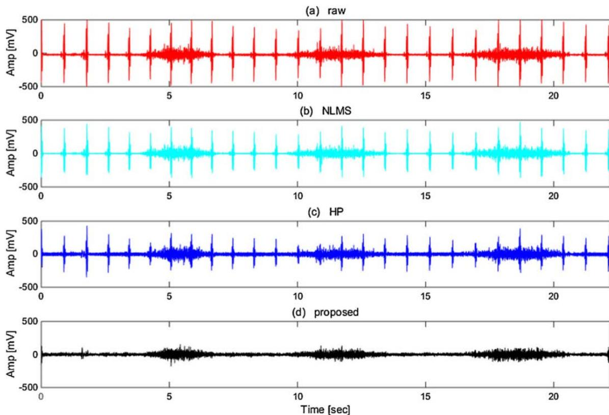
Figure 20 EMGdi signal denoising outputs comparison: (a) Raw EMGdi signal (b) Normalized least mean square filter (c) High pass filter (d) ICA—wavelet filter (Wu, Tong & Yang 2016)
