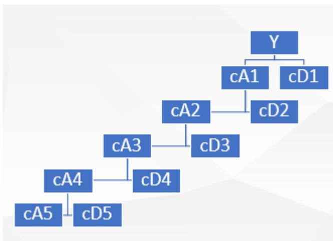
Figure 6 Structure of five-layer multi-resolution analysis
