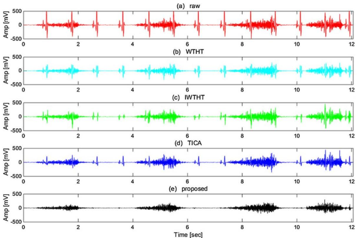
Figure 19 EMGdi signal denoising outputs comparison: (a) raw EMGdi signal (b) hard thresholding filter (c) inverse hard thresholding filter (d) traditional ICA filter (e) ICA—wavelet filter (Wu, Tong & Yang 2016)
