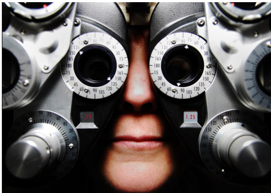
Figure 4.1 Optical Phoropter (U.S. Navy, 2010. Public Domain).
