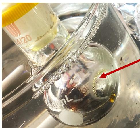
**B** Receiving flask under 15 mbar at 170 °C
