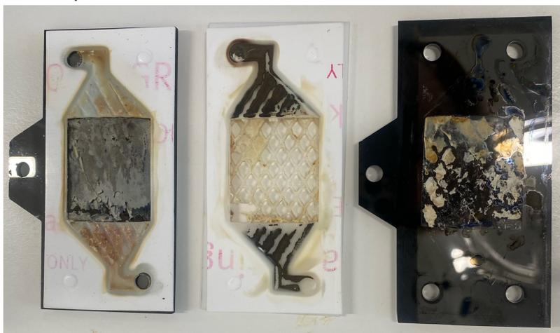
**B** Polymer build after a flow rate of 2 mL/min
