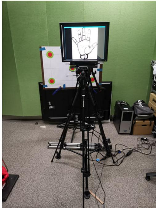
Figure 6.2: Recording setup with Microsoft Kinect 2.0 and a computer monitor set up on tripods. A Intel RealSense D435i is also mounted on the tripod in this image: this was purely for interest and served no functional purpose.
