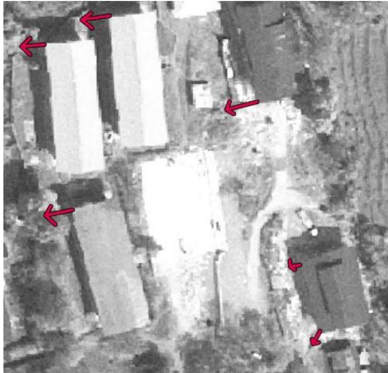
Figure 15. The arrow representing the alignment error of Panchromatic imagery with the base imagery
