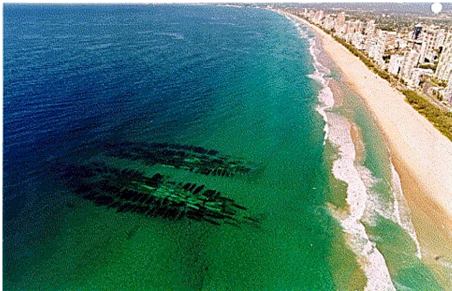
Figure 12: The Artificial Surf Break in Gold Coast, Queensland (AU). The artificial reef presents a “V” shape, with the apex pointing seaward. Source: Courtesy of the International Coastal Management, Australia, www.coastalmanagement.com.au (Ranasinghe and Turner, 2006) Reproduced with permission.
