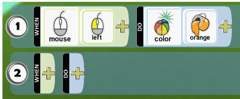
Figure 4.21: Two Kodu rules captured within Kodu Game Studio (Microsoft Corporation (Research), 2017). Rule 1 is complete and describes changing an object's colour to orange when left-clicked with a mouse. Rule 2 is empty.
