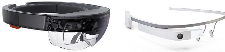
Figure 2.2: Microsoft HoloLens (left) provides a stereoscopic view via twin optical combiners. The Google GLASS headset (right) provides a monoscopic view via a small projector mounted above the right eye.
