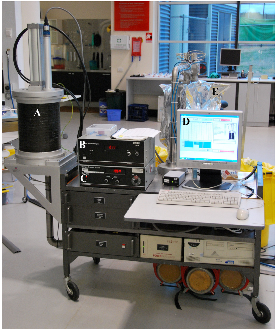
Plate 4-2: The laboratory-based Maximum Oxygen Uptake System electronic (MOUSE) indirect calorimetry system, including: A) volume piston; B) AEI Technologies CD-3A CO 2 gas analyser; C) AEI Technologies S-3AI O 2 analyser; D) computer interface, and E) Mylar Douglas bags.
