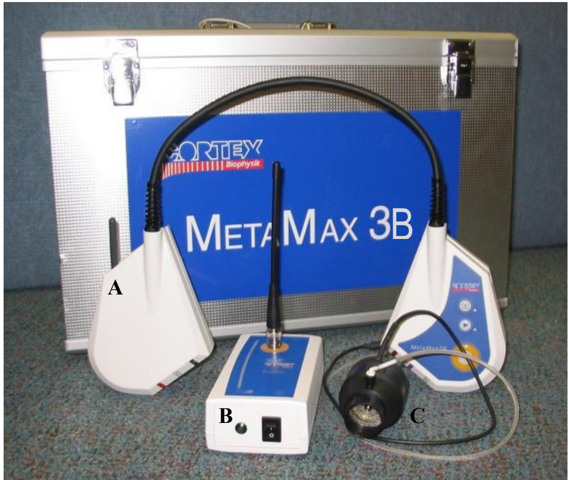
Plate 4-1: The MetaMax3B portable indirect calorimetry system, including: A) gas analysis-data telemetry module; B) telemetry receiver unit, and C) volume turbine assembly.
