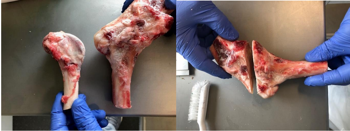
Figure 3.1: A representative sample of (a) frozen ovine distal femoral condyle before cutting (b) distal femoral condyle with the top soft tissue and cortical bone cut off
