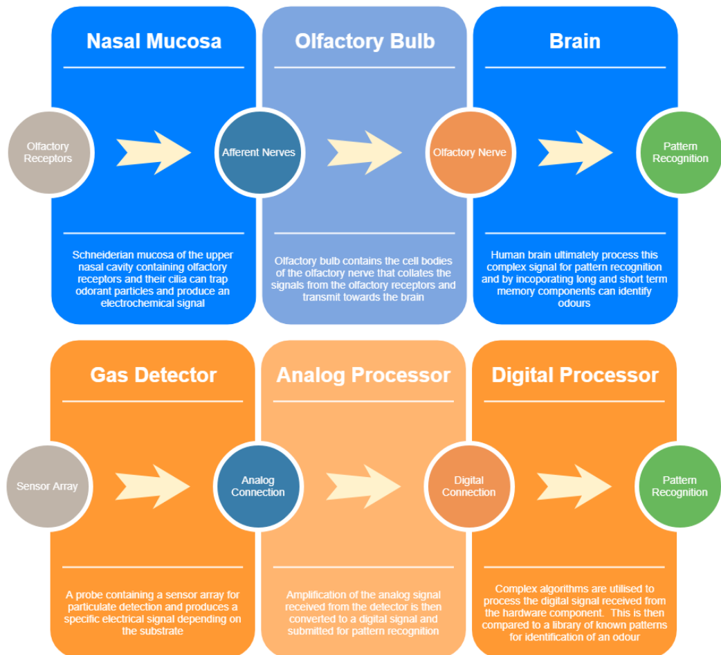
Figure 35. Comparison of human olfactory system to E-Nose.
