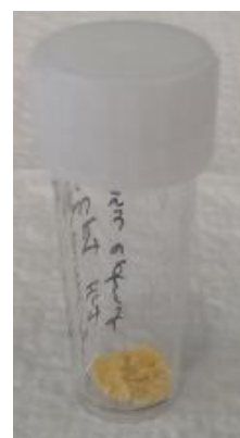
Figure 4-18: Dried precipitate from secondary liquid/liquid extraction of C. officinalis SCF residue using aqueous NaOH
