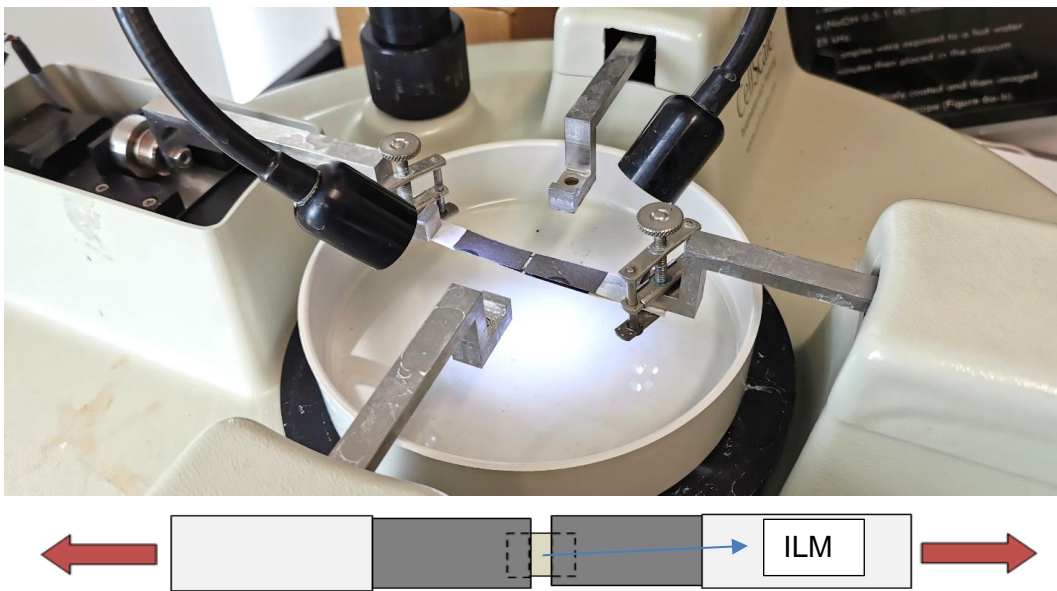
Fig. 12 The specimen prepared was loaded on the cellscale device for micromechanical testing in tensile direction.
