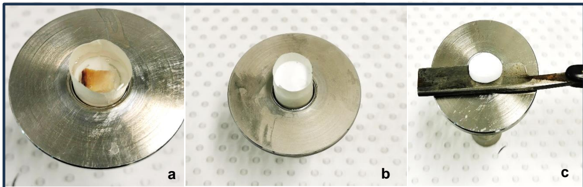
Fig. 7 The specimen is set at -20^{\circ}\text{C} (b) with OCT fluid filled in it (a). A feather blade (c) was used to slice the specimen measuring 1mm height.
