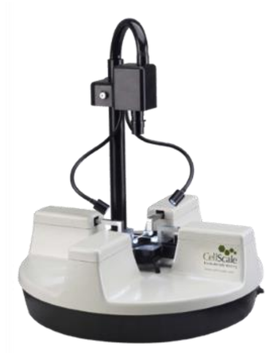
Fig. 13 CellScale micromechanical testing device used for uniaxial testing
