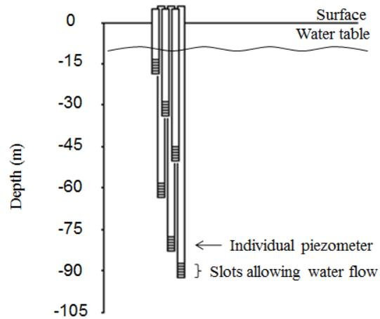
**Figure 2.1** Schematic of the 6 individual (50 mm diameter) piezometers installed as a nest at Ashbourne, South Australia. The water table is found approximately 8 m from the surface. The slot depth for each individual piezometer covers approximately 5 m.
