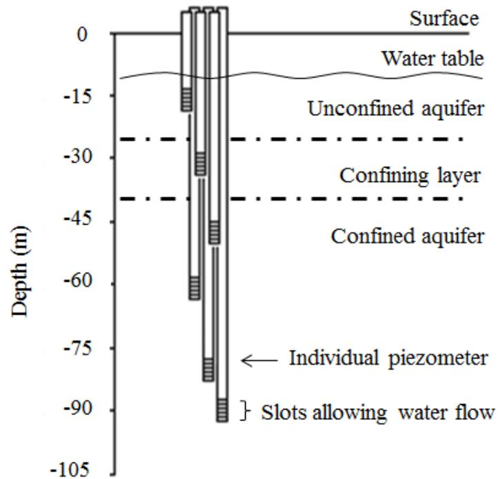
**Figure 4.1** Schematic representation of the Ashbourne nested piezometer consisting of six, 50 mm diameter, individual PVC piezometers installed as a nest. The water table is approximately 8 m beneath the soil surface. Each piezometer had a slot/screen length of approximately 5 m, at the following depths: 13–19 m (the unconfined aquifer), 29–34 m (the confining layer) and 42–47, 58–63, 79–84, 87–92 m (the confined aquifer).
