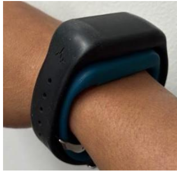
Figure 10 Axivity AX6 sensors worn on top of each other at right wrist for sampling rate comparison
