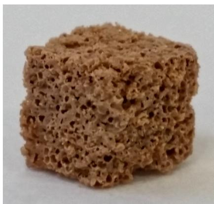
**Figure 4.1.2** | Cube of porous polysulfide, approximately 5.0 mm across on each side.
