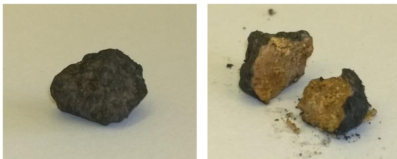
**Figure 3.1.6** | Canola oil polysulfide. Left: single pellet after treatment with Hg<sup>0</sup>, right: same pellet cracked open. The polysulfide only alters colour at the surface.
