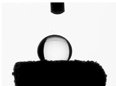
Water droplet on cube of porous polymer
