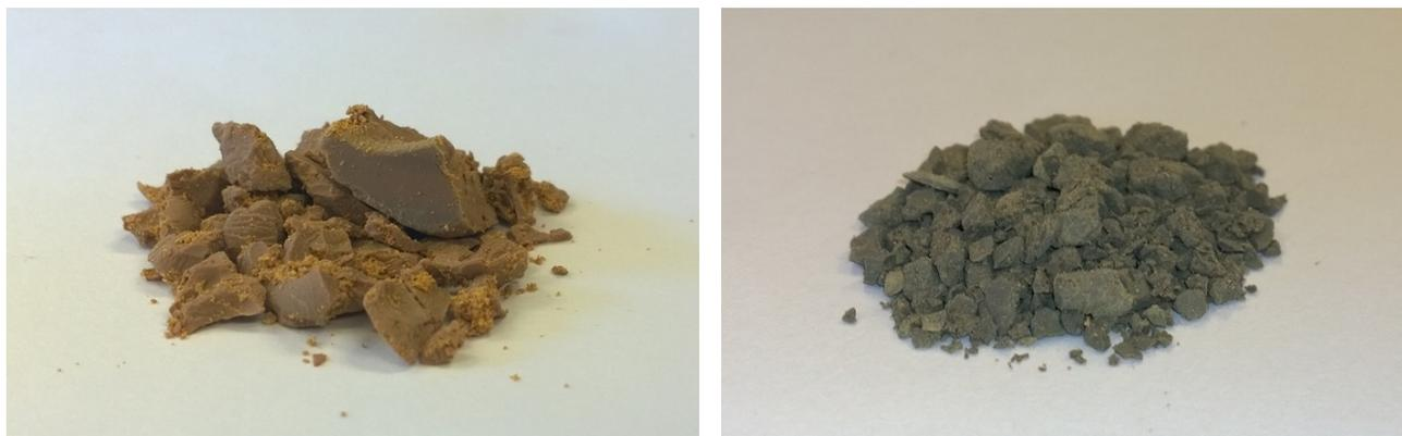
**Figure 3.1.1** | Canola Oil Polysulfide. Left: as synthesised using standard procedure, right: after treatment with HgCl<sub>2</sub> (20 mg mL<sup>-1</sup>, 24 hours). The material has turned from brown to grey.
