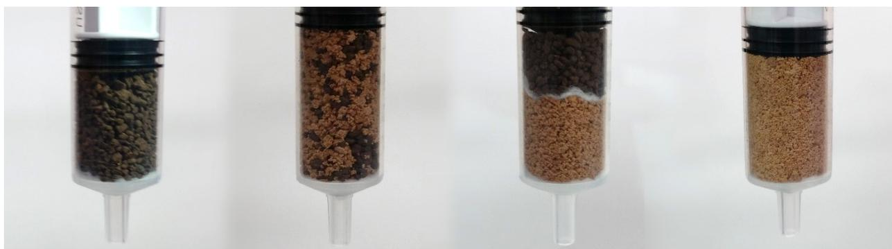
**Figure 3.1.42** | Photo of columns before use. Left to right: Soil only, soil and polymer mixed together, soil and polymer layered with cotton wool, polymer only.
