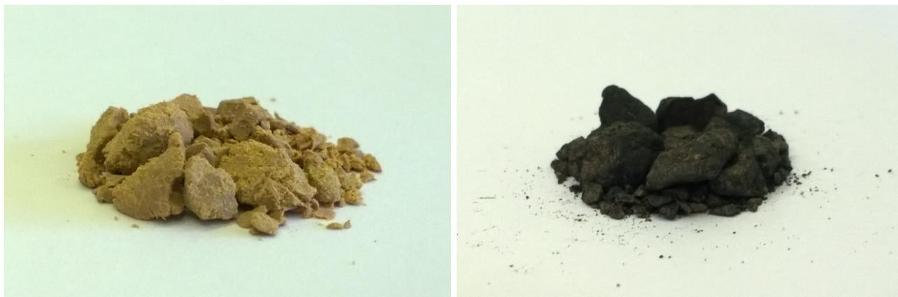
**Figure 3.1.5** | Canola oil polysulfide. Left: as synthesised using standard procedure, right: after treatment with Hg<sup>0</sup> (170 mg mercury, 2.0 g polysulfide, 24 hours). The material has turned from brown to black.
