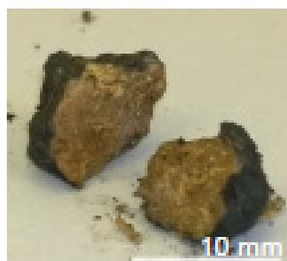
**Figure 3.1.15** | The surface of the canola oil polysulfide (50 % sulfur) reacts with mercury metal, forming a black product. EDS analysis verifies mercury is found on the surface of the material.
