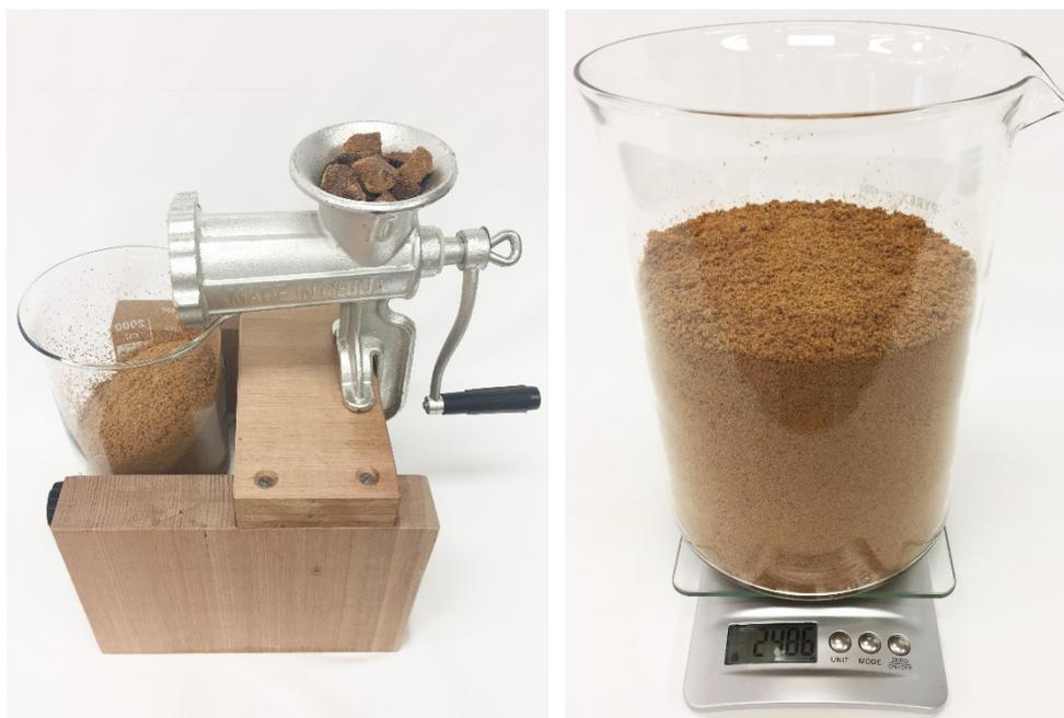
**Figure 2.1.55** | The canola oil polysulfide salt composite is a friable rubber, easily processed into particles using a mechanical grinder.
