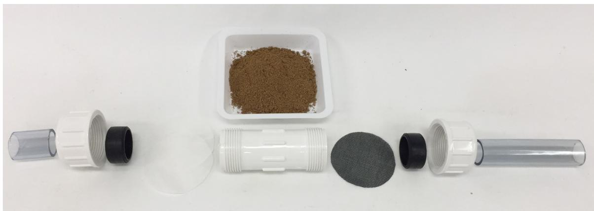
**Figure 4.1.20** | Components for a filtration apparatus used to separate crude oil and seawater.
