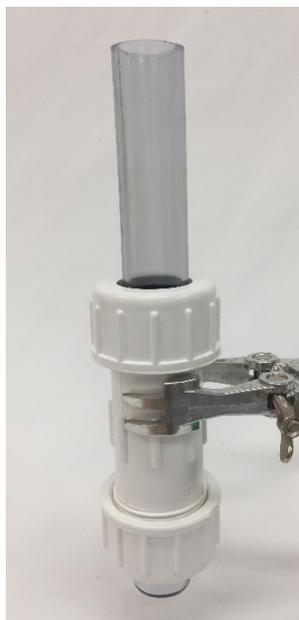
**Figure 4.1.21** | Assembled filtration apparatus used to separate crude oil and seawater.
