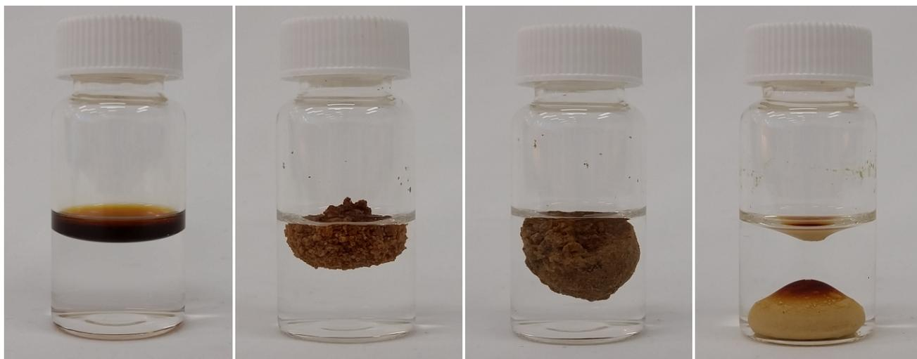
**Figure 4.1.24** | From left to right – Nockatunga crude oil on water; porous polymer added to oil; non-porous polymer added to oil; sulfur added to oil.
