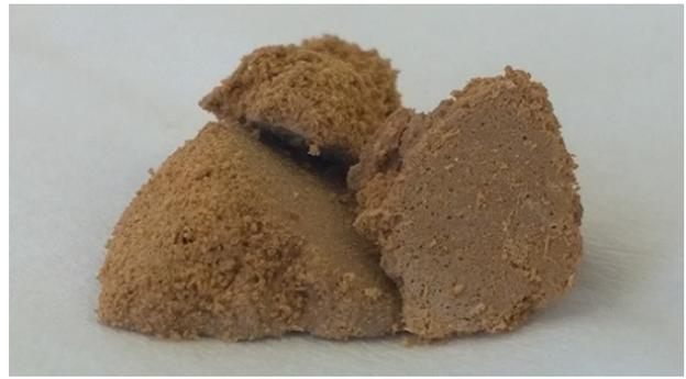
**Figure 2.1.42** | Left: polymer before wash procedure, right: polymer after wash procedure
