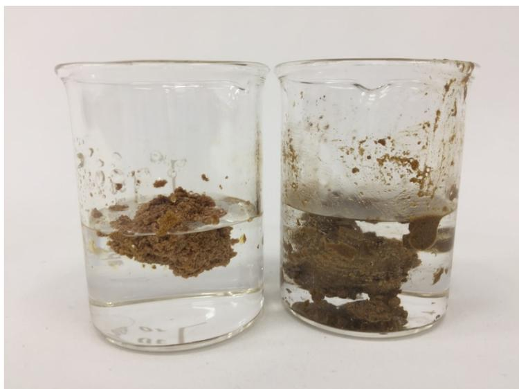
**Figure 4.1.25** | Left: Only 1.15 g of the low density canola oil polysulfide was required to capture the 2.00 g crude oil. The particles aggregate upon sorption of the oil and float on the water. Right: non-porous canola oil polysulfide particles still bind to crude oil and aggregate, with 2.96 g of polymer required to bind all oil. The non-porous polymer and oil product does not float on water.
