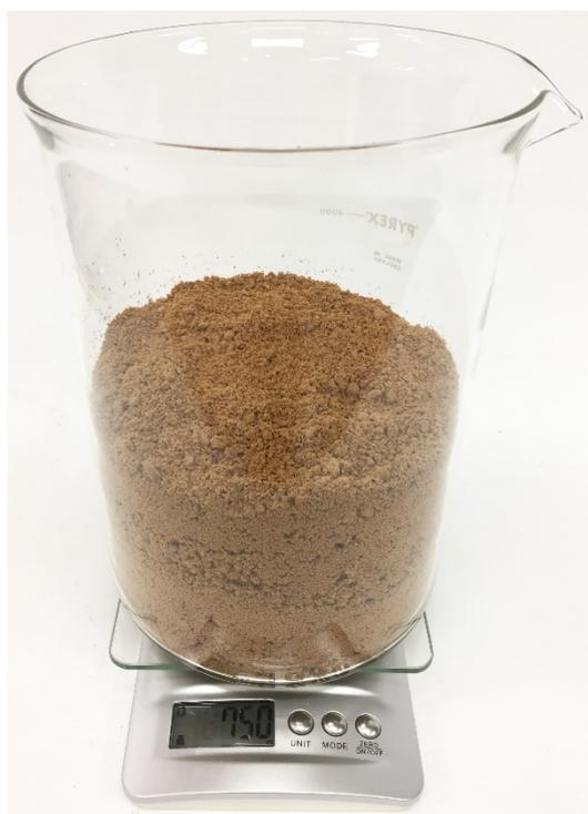
**Figure 2.1.56** | Washed and dried porous canola oil polysulfide, prepared on a 750 g scale.
