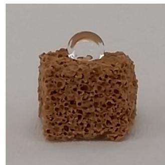
10  $\mu$ L droplet on 0.5 cm-side cube of polysulfide
