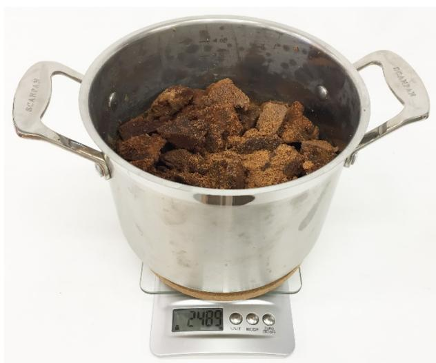
**Figure 2.1.54** | The canola oil polysulfide and salt composite, after breaking down into large pieces with a spatula or paint scraper.
