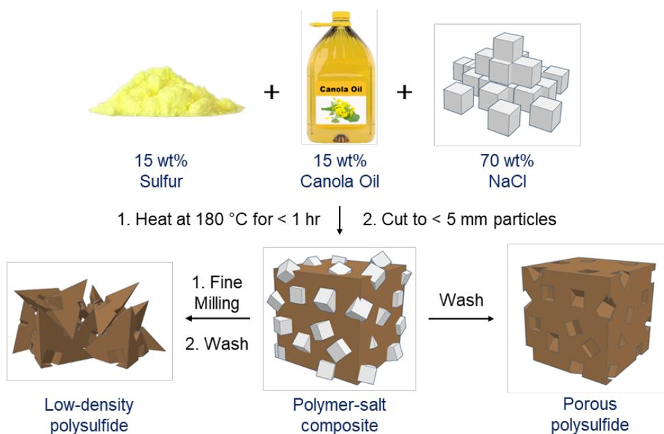
**Figure 2.15** | Illustrative diagram of porous and low-density polysulfide synthesis.
