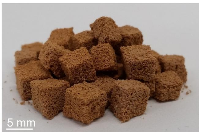
**Figure 2.1.49** | Approximately 5.0 mm-side polysulfide cubes
