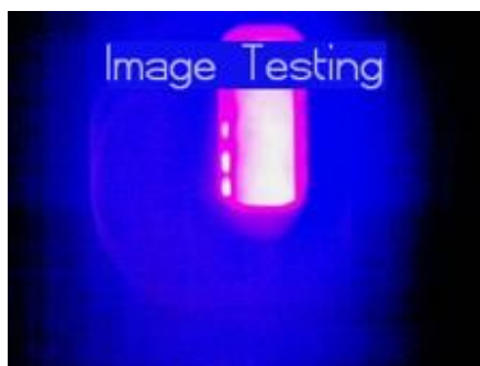
Figure 4.3: The fluorescence signal from the TPE powder was over the detection range of the camera, causing the saturation in the obtained image.
