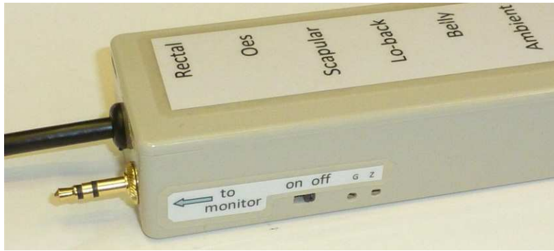
(C) The sensor connector box showing the location of the on-off switch and gain and zero adjustments that allowed use with several brands of patient monitor.
