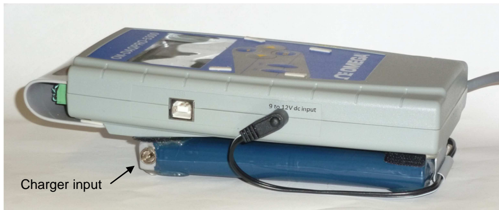
Figure B2. An extension battery in situ beneath the datalogger An Omega datalogger is pictured above an external extension battery.
