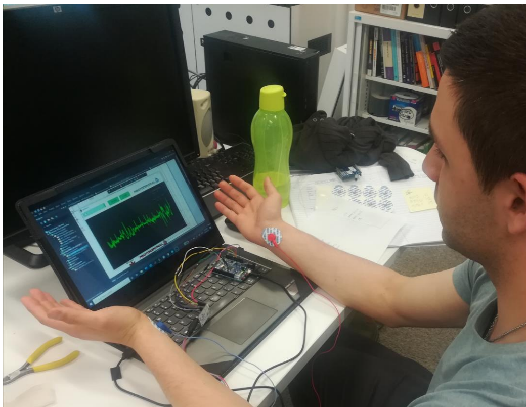
Figure 12: I connected myself to the circuitry and successfully obtained an ECG signal
