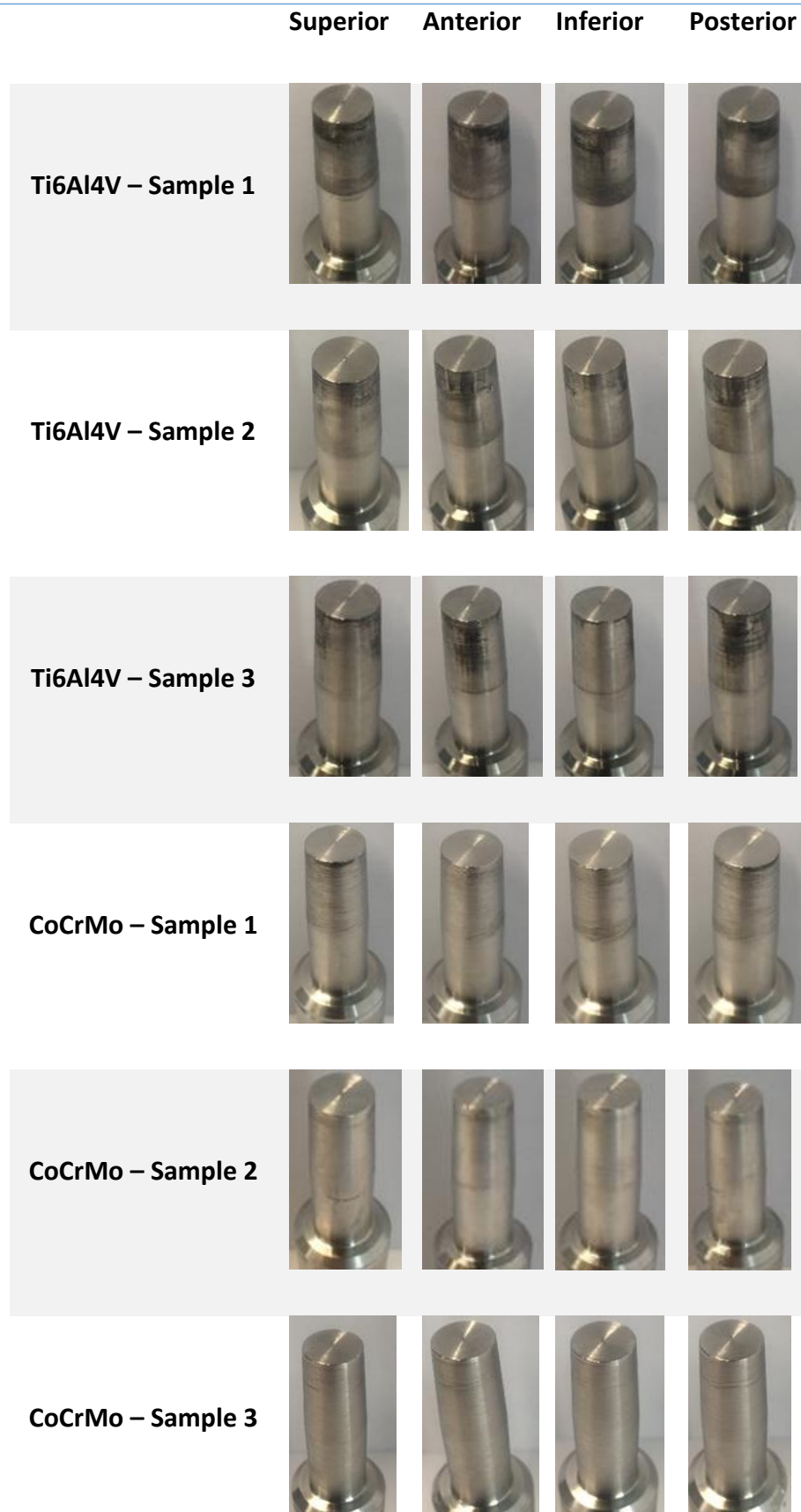
Figure 6.9 Ti alloy and CoCr alloy neck samples fretting-corrosion damage after undergoing cyclic loading test in corrosive medium
