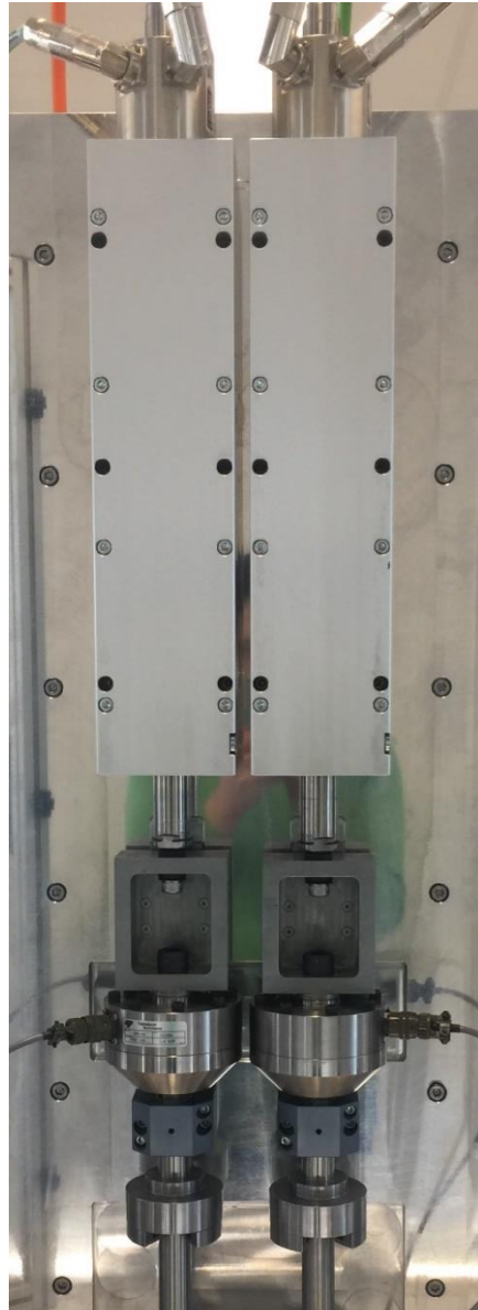
Figure 5.7 Two linear direct drive motors mounted in parallel inside cooling flanges for cooling of the motor through circulating chilled water through flanges
