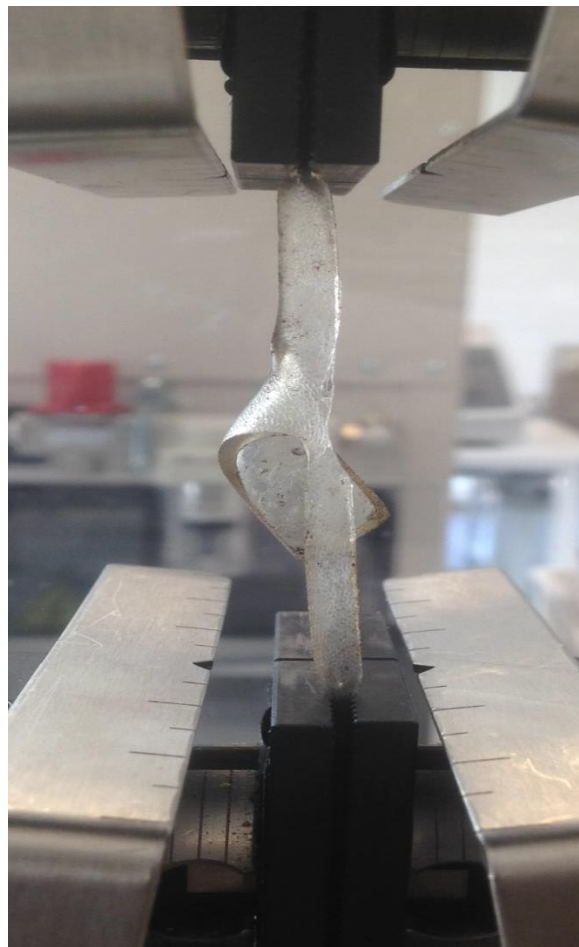
Figure 41 Uneven propagation of crack from notch
