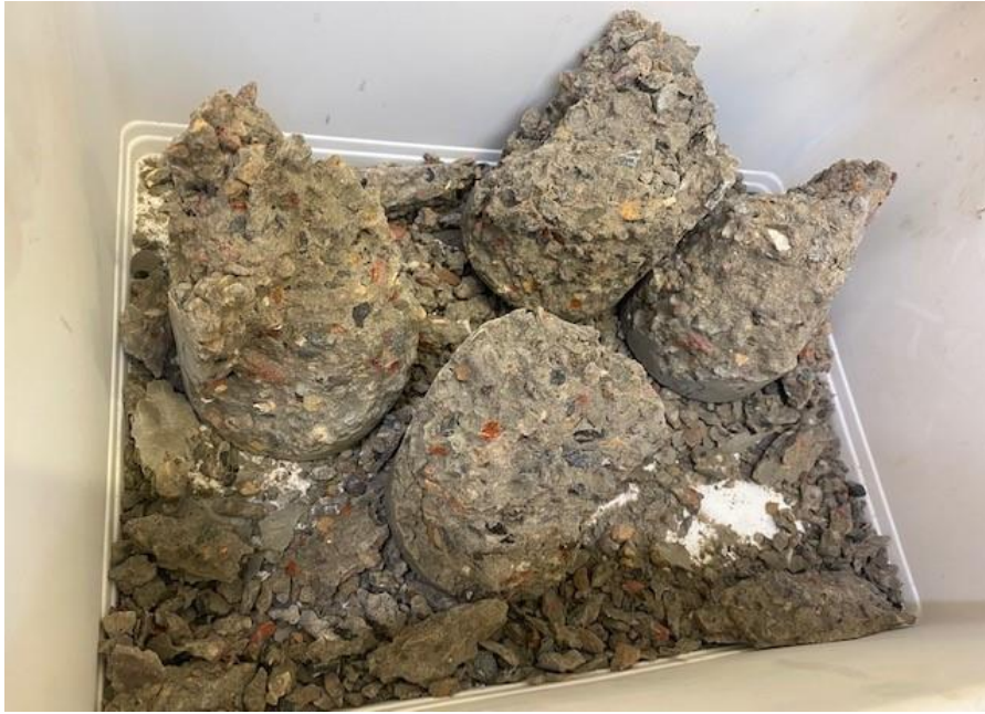
Figure 39: Two cylinders tested on 7th day for compressive strength
