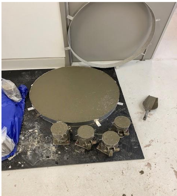
Figure 48: Resting for 24 hrs to get a harder concrete
