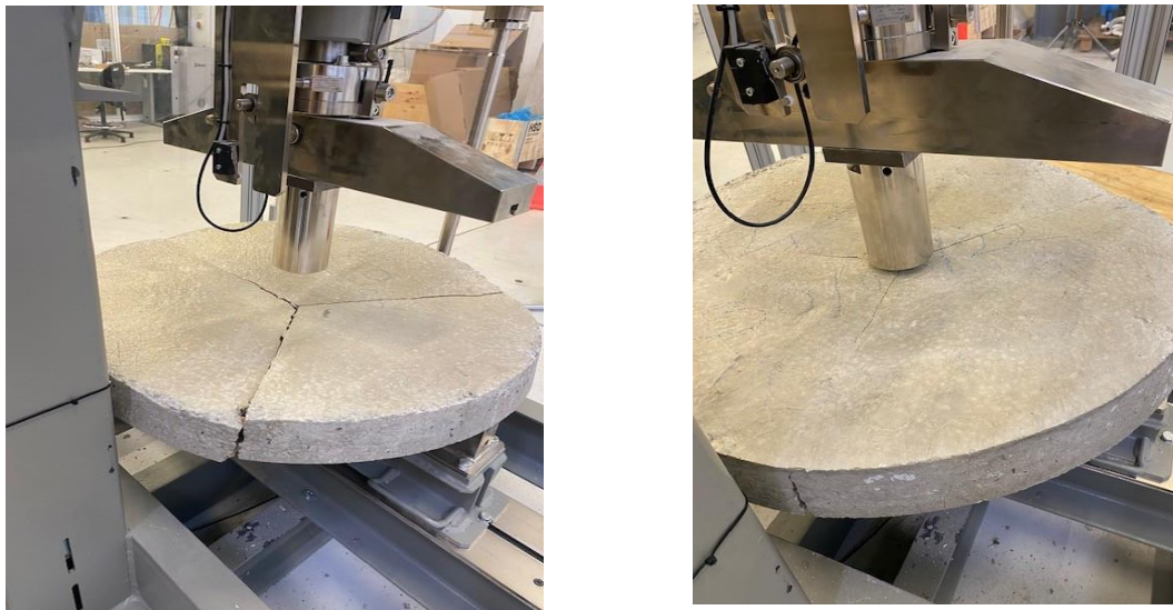
Figure 28: An upper view of the failure of the control mix panel (left) and failure of the Toberite concrete panel (right).
