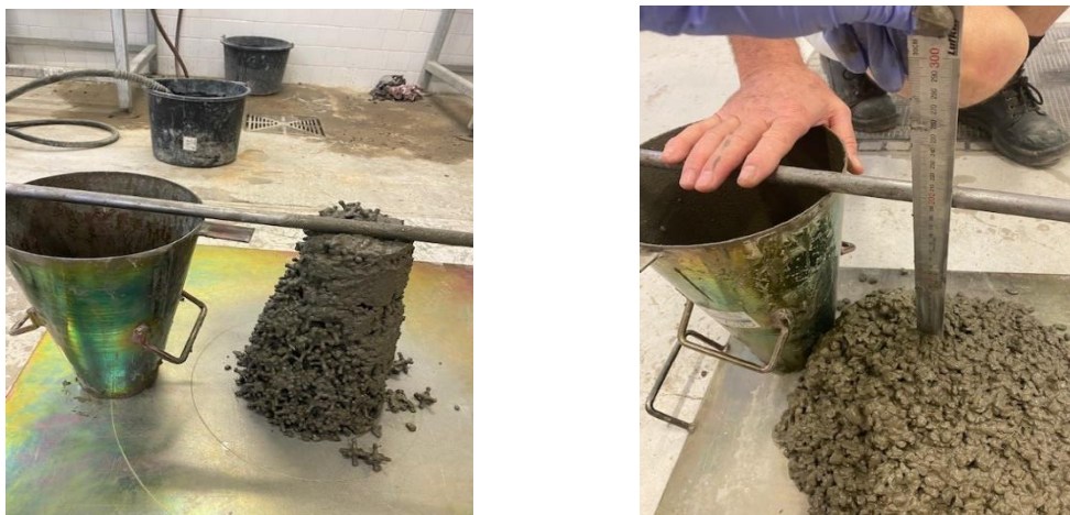
Figure 27: Slump test for 50% Toberite (left) and for 0% Toberite (right)
