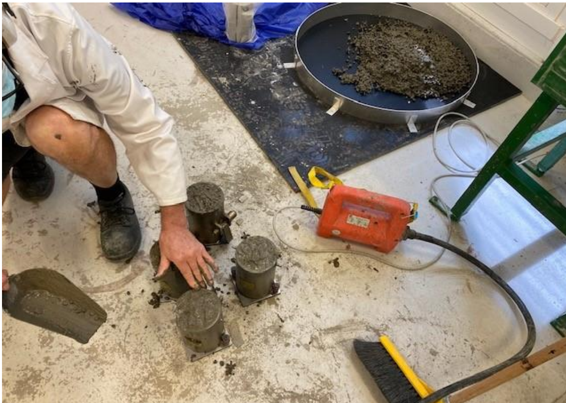
Figure 34: Fill up the moulds
