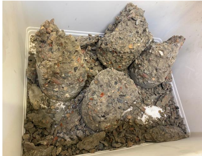
Figure 15: Concrete specimen after failure
