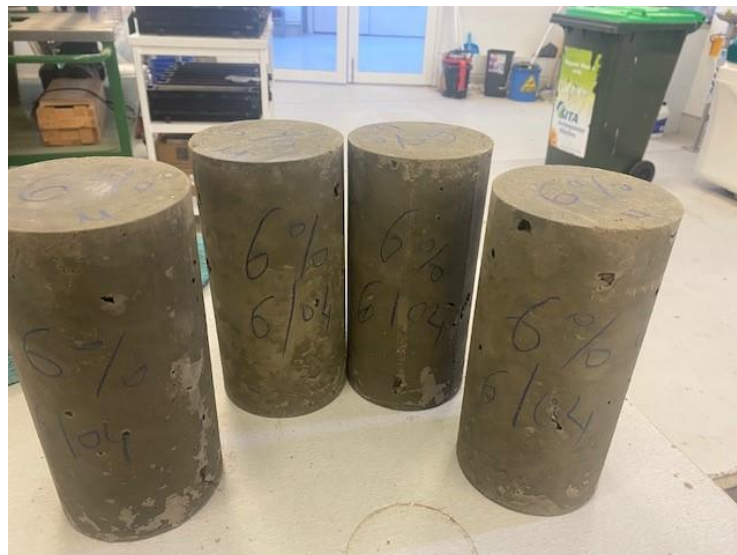
Figure 18: Air voids in the cylindrical sample
