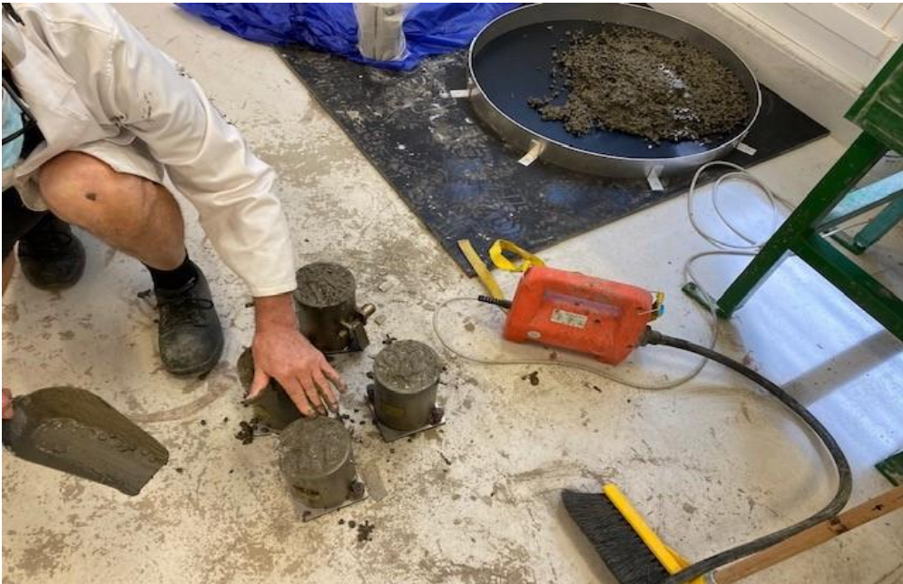
Figure 50: Filling the moulds
