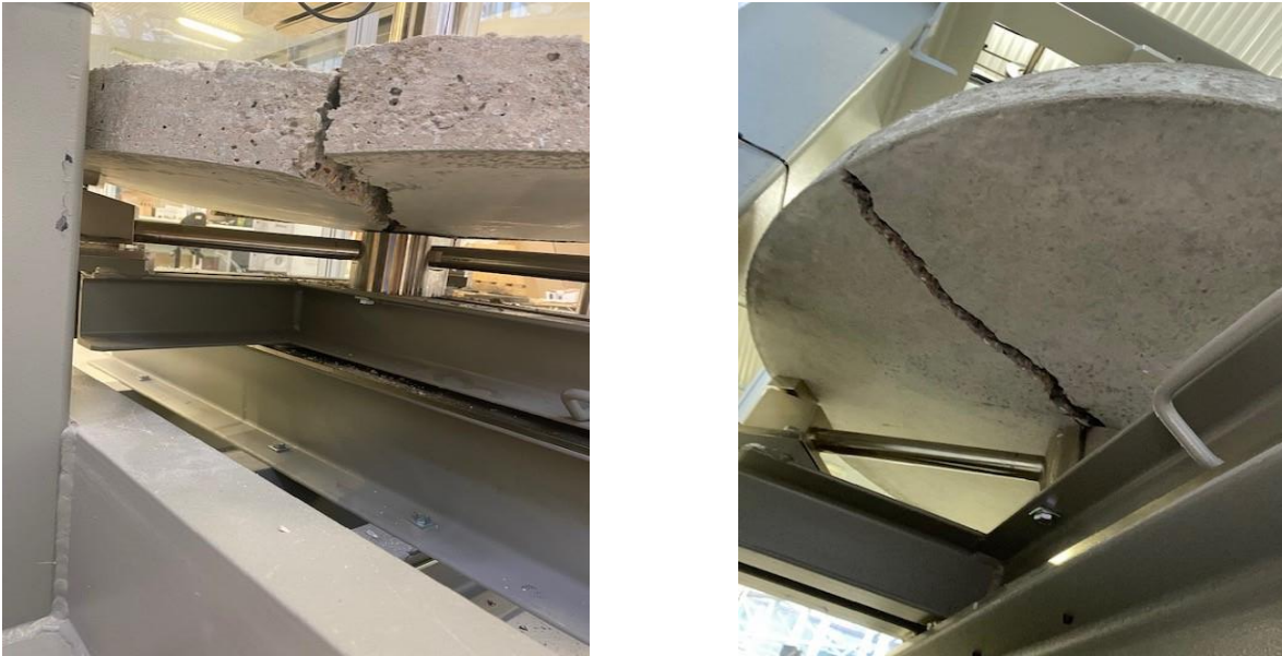
Figure 29: A downer view of the failure of the control mix panel (left) and failure of the Toberite concrete panel (right).
