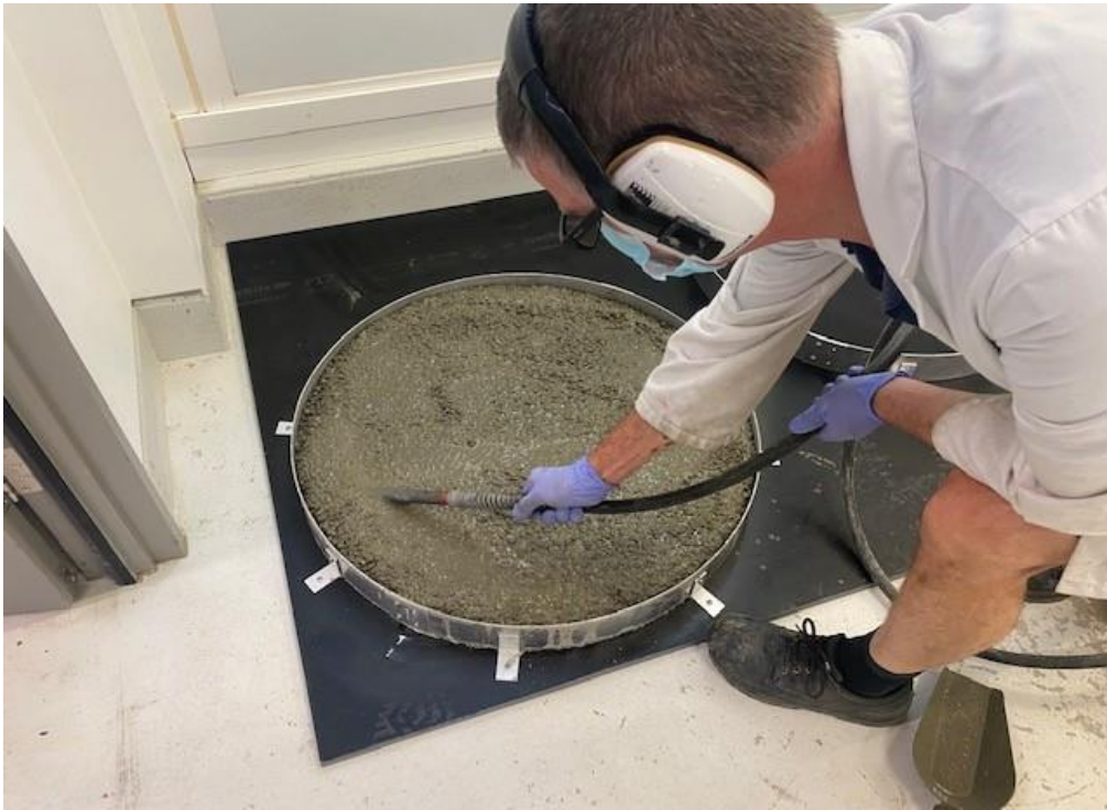
Figure 35: Vibrating the panel
