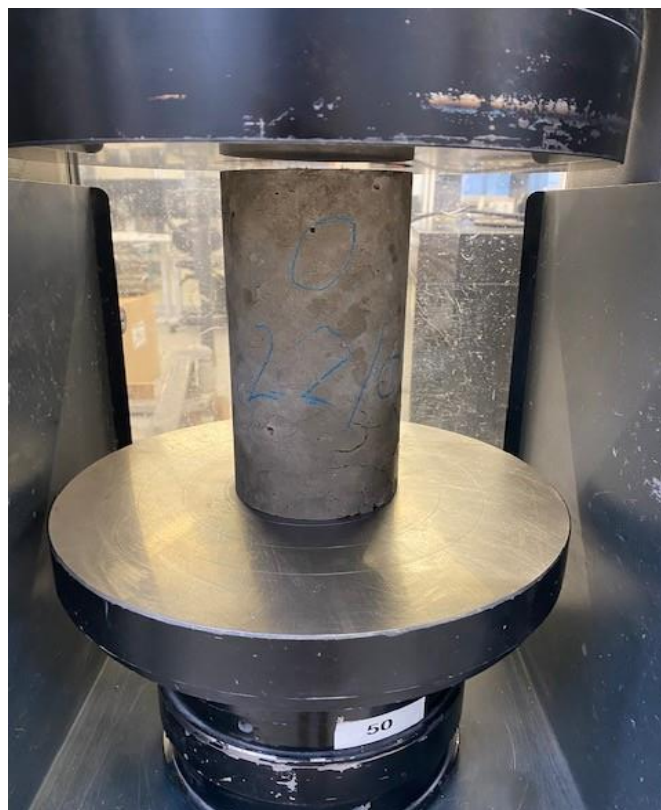
Figure 38: Compressive Strength test on 7th day
