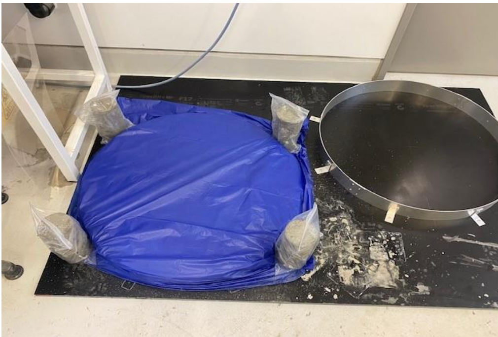
Figure 42: Cover of the moulds with plastic sheets
