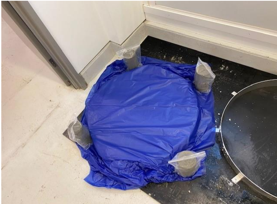
Figure 37: Cover with plastic sheet for the evaporation aim
