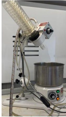
Figure 1: The main body of the extraction equipment consists of a round-bottomed flask, a reflux condenser tube and a water bath heating device.
