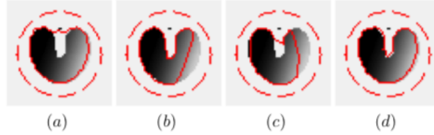
Figure 4: Comparison using image with U-shaped gradient object. A snake convergence to concave regions, (a) with the VFC which is easily affected by noise, (b) Chan-Vese snake, the contour leaks through the right side with weak boundary information, (c) RAGS, the contour leak through the right side of the U shape even the noise is so small that it is merged into the background, and (d) VFCCV, the contour converges to the correct U-shape boundary and is robust to the noise. Sourced from [25].
