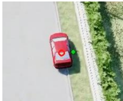
Figure 14. True (red) and measured (green) object bounding box centre with vehicle facing North (bottom-to-the-top)
