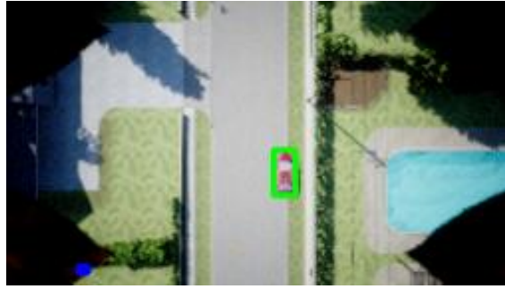
Figure 10. Image taken from Airsim camera with manually identified object bounding box
