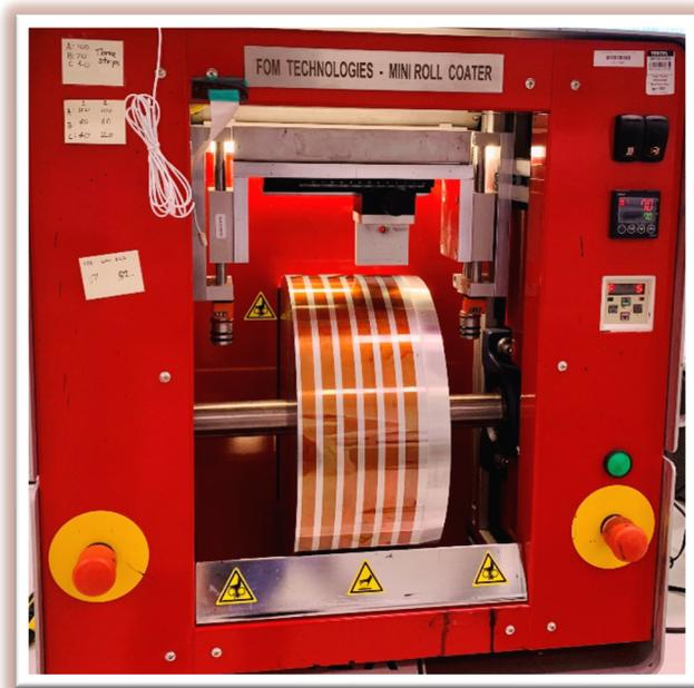
**Figure 5.16:** FOM Mini-roll coater used for printing of polymer solar cells.
