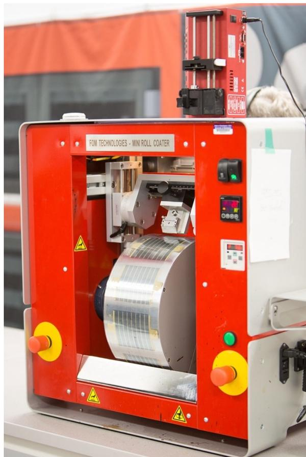
**Figure 5.2:** Mini-roll coater (FOM Technologies).
